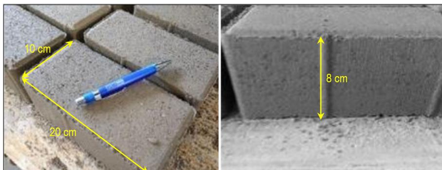
**Figure 5.** Visual aspect of the block produced using iron-ore sand.
