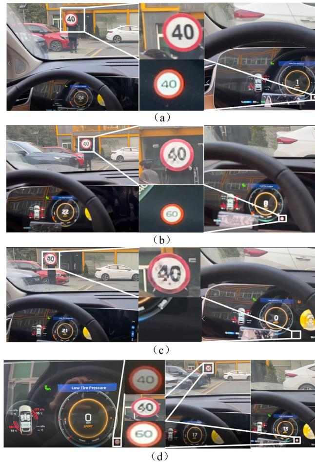
**Figure 10.** Camera attack based on adversarial examples: (a) no attack; (b) no target attack; (c) target hide attack; (d) specific target attack.
