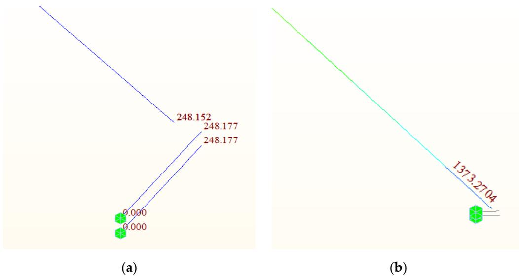
**Figure 10.** Steel beam rigid joint simulation. (a) Vertical displacement. (b) cable force.
