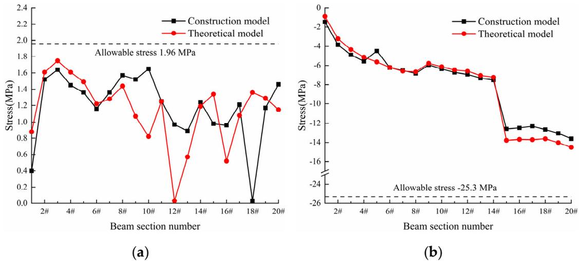
Figure 13. Bridge deck panel stress during construction phase. (a) Tensile stress. (b) Compressive stress.
