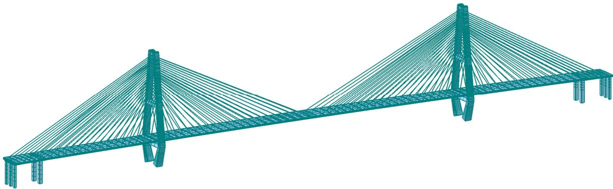
**Figure 3.** Spatial finite element model of the Xiangsizhou Bridge.
