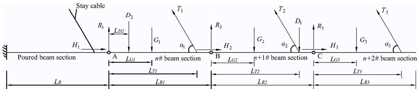
Figure 12. Force diagram of three-segment cyclic structure.
