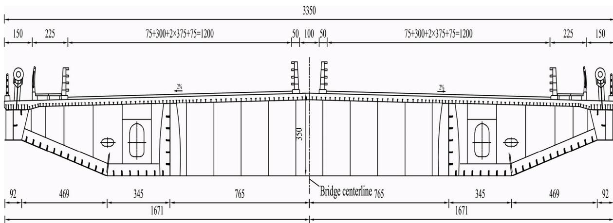
Figure 2. Cross-section of the main girder of The Xiangsizhou Bridge (unit: cm).
