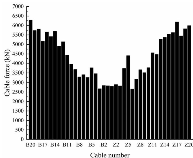
Figure 8. Cable force distribution at reasonable completion state.
