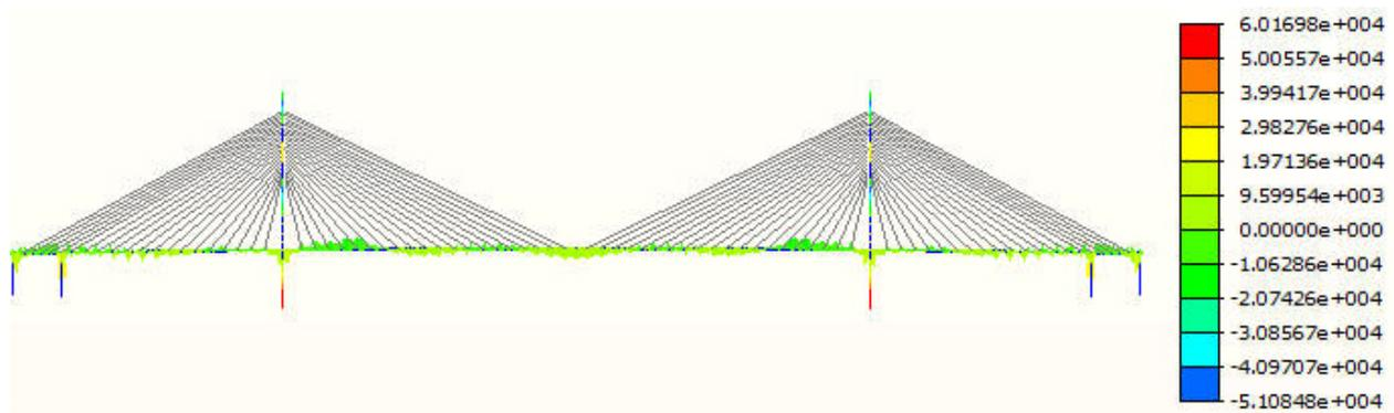
Figure 6. Bending moment of the Xiangsizhou Bridge (unit: kN·m).
