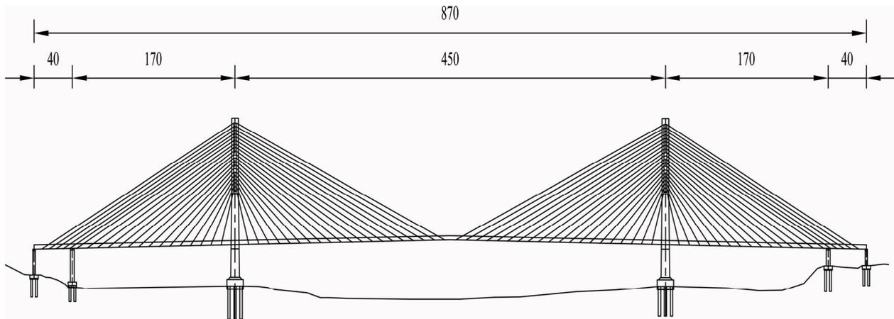
Figure 1. Arrangement of the main bridge of The Xiangsizhou Bridge (unit: m).
