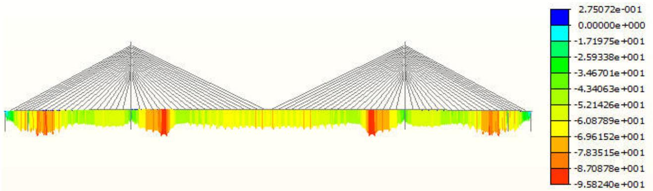
Figure 7. Stress in the main girder of the Xiangsizhou Bridge (unit: MPa).
