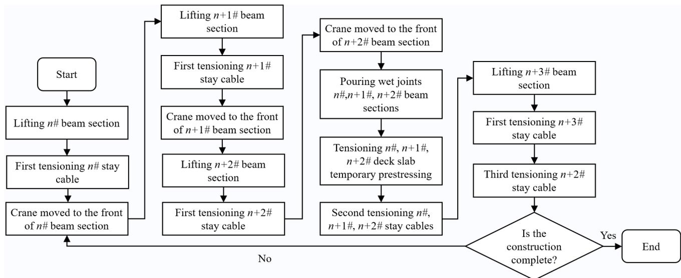
**Figure 9.** Three-segment cycle construction steps.
