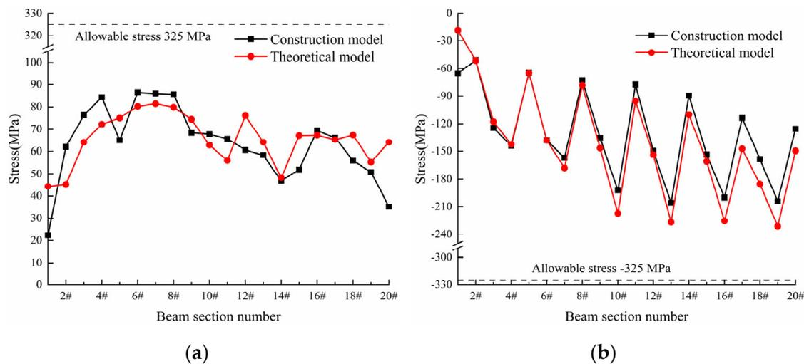
Figure 14. Steel main beam stress during construction phase. (a) Tensile stress. (b) Compressive stress.
