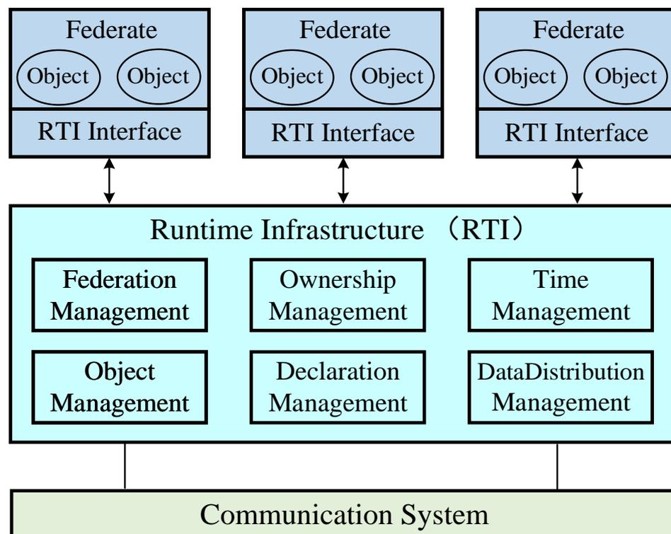
Figure 3. Construction of the federation in an HLA.
