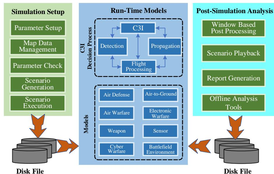
Figure 7. EADSIM architecture.
