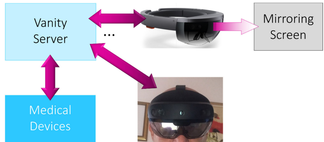
Figure 8. VanityX platform supporting multiple HoloLens2 headsets.
