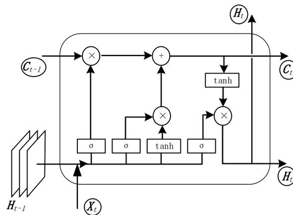
**Figure 3.** LSTM cell structure diagram.
