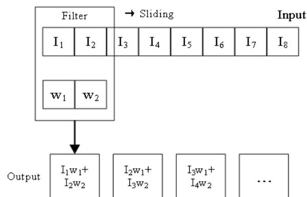
Figure 2. Schematic diagram of one-dimensional convolution algorithm.
