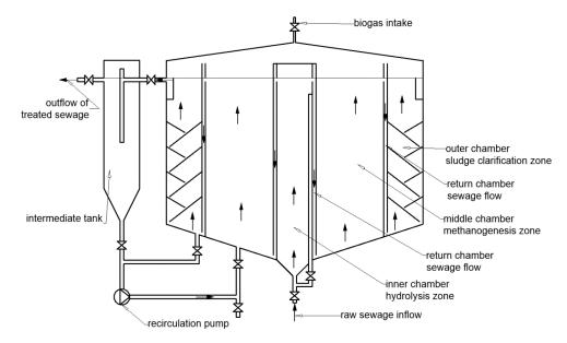
Figure 1. Scheme of anaerobic labyrinth-flow bioreactor.
