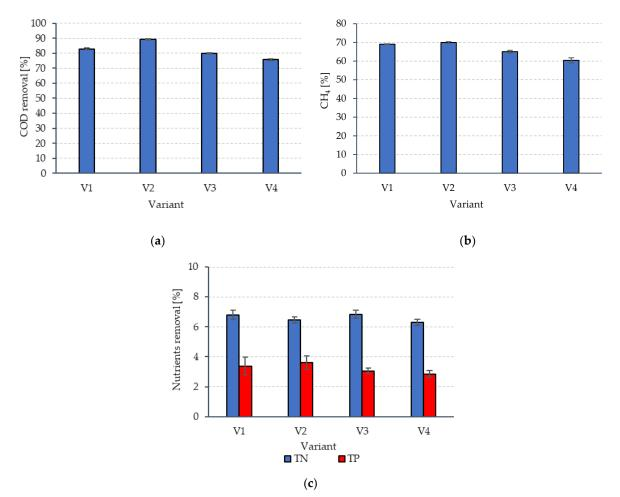
**Figure 5.** The efficiency of anaerobic dairy treatment in stage 2: (a) organic compound removal as COD with a standard deviation in experimental variants V1–V5; (b)  $CH_4$  concentration in biogas with a standard deviation in experimental variants V1–V5; (c) nutrient removal (nitrogen and phosphorus) with a standard deviation in experimental variants V1–V5.
