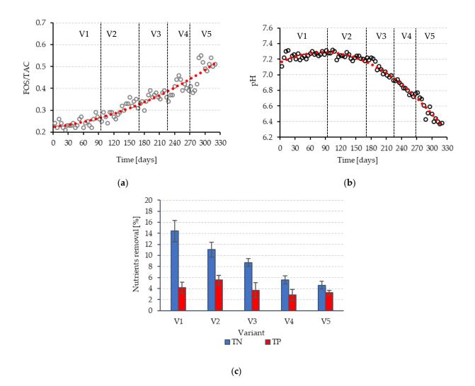
**Figure 3.** The efficiency of anaerobic dairy treatment in stage 1: (**a**) FOS/TAC ratio in the methanogenesis tank during the experimental time (variants V1–V5); (**b**) pH in the methanogenesis tank during the experimental time (variants V1–V5); (**c**) nutrient removal (nitrogen and phosphorus) with a standard deviation in experimental variants V1–V5.
