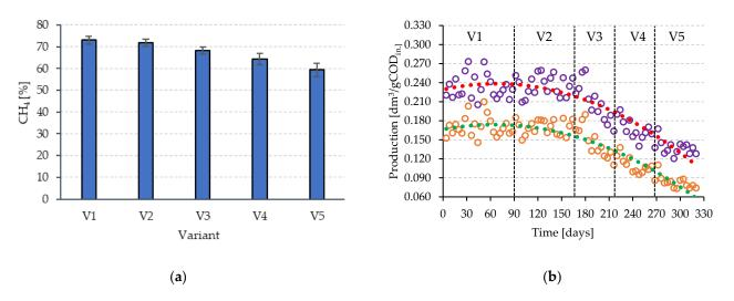
**Figure 4.** The efficiency of anaerobic dairy treatment in stage 1: (a)  $CH_4$  concentration in biogas with a standard deviation in experimental variants V1–V5; (b) biogas and methane yield per gram of COD inlet during the experimental time (variants V1–V5).
