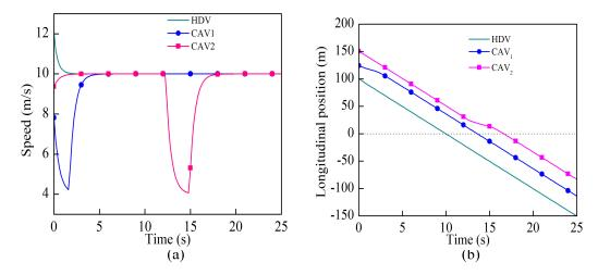
**Figure 6.** The speed and position curves of all the vehicles during the whole crossing; (**a**) the speed, (**b**) the position.
