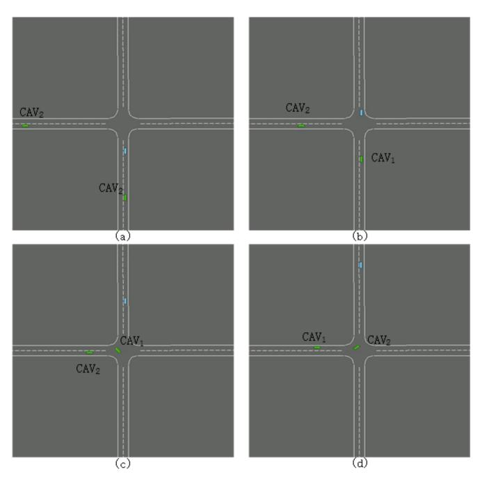
**Figure 7.** The frames of the time slices showing the interactions performed by the simulation platform (blue: HDV; green: CAVs); (**a**) 9 s, (**b**) 12 s, (**c**) 15 s, and (**d**) 18 s.
