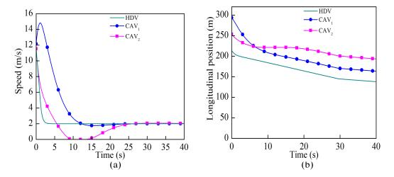
**Figure 11.** The speed and position curves of all the vehicles when the HDV traveled at a low speed using the heuristic rule-based algorithm; (**a**) the speed, (**b**) the position.
