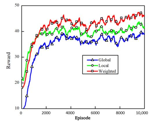
on an agent's location. The weight reward assignment scheme assigned more rewards to the vehicles closer to the intersection, which facilitated the cooperation between the agents.
