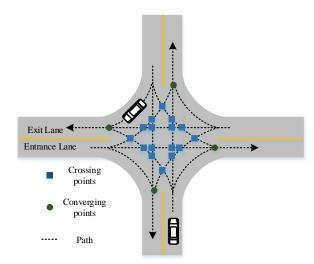
Figure 1. Illustration of the considered single-lane four-way unsignalized intersection scenario.
