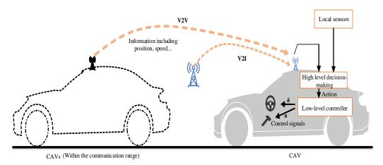
Figure 2. Schematic diagram of the decision control for multiple intelligent vehicles.
