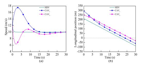
**Figure 10.** The speed and position curves of all the vehicles in the ideal traffic using the heuristic rule-based algorithm; (**a**) the speed, (**b**) the position.
