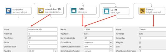
**Figure 14.** Representation of the hybrid model with CNN and LSTM layers.
