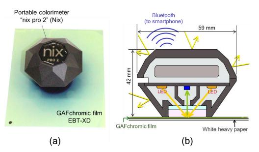
**Figure 1.** The materials used for this study (**a**): Gafchromic film "EBT-XD" and a portable colorimeter "nix pro 2" (abbreviated to "Nix" here) and a cross-section drawing of Nix (**b**). The black frame structure of Nix blocks well the ambient light; two LED sources (orange part) cast light beams and a color sensor (blue part) detects the reflected light; the data of color intensities measured as RBE and CMYK components are transferred to a smartphone via Bluetooth.
