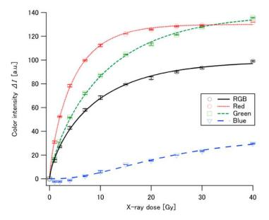
**Figure 3.** Dose dependences of the color intensities of EBT-XD irradiated with 160 kV X-rays at up to 40 Gy as to RGB, red, green and blue components measured with Nix at the angle of  $0^{\circ}$ .
