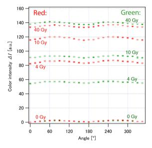
**Figure 4.** Angle dependences of the color intensities as to the red and green components of EBT-XD measured with Nix with 15° intervals after irradiation with 160 kV X-rays at 0 (control), 4, 10 and 40 Gy.
