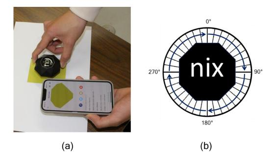
**Figure 2.** A scene of reading the EBT-XD film using Nix (**a**) with a smartphone application for reading exclusively the data from Nix via Bluetooth. The measurements of the films in a few hours after irradiation with 160 kV X-rays. Angle dependence of measured color intensities was examined by rotation of Nix with 15° intervals in a clockwise direction (**b**).
