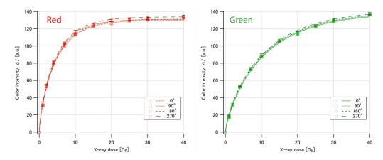
**Figure 5.** Dose dependence of the color intensities (**left**): red component, (**right**): green component) of EBT-XD irradiated with 160 kV X-rays at up to 40 Gy and measured with Nix at four angles: 0°, 90°, 180° and 270°.
