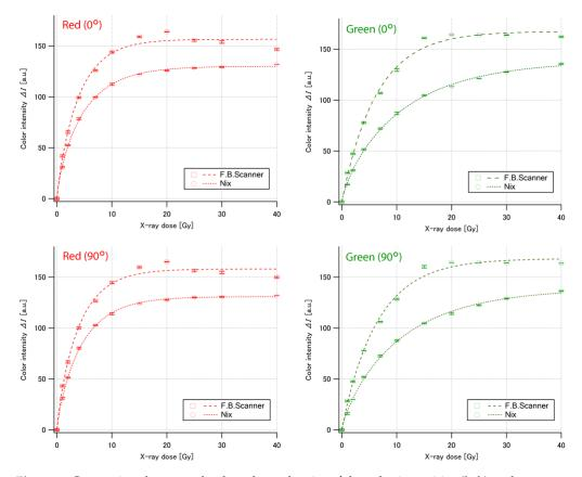
**Figure 6.** Comparison between the dose dependencies of the color intensities (**left**): red component, (**right**): green component) of EBT-XD measured with Nix and those with the flatbed scanner at the angles of  $0^{\circ}$  (**above**) and  $90^{\circ}$  (**below**).
