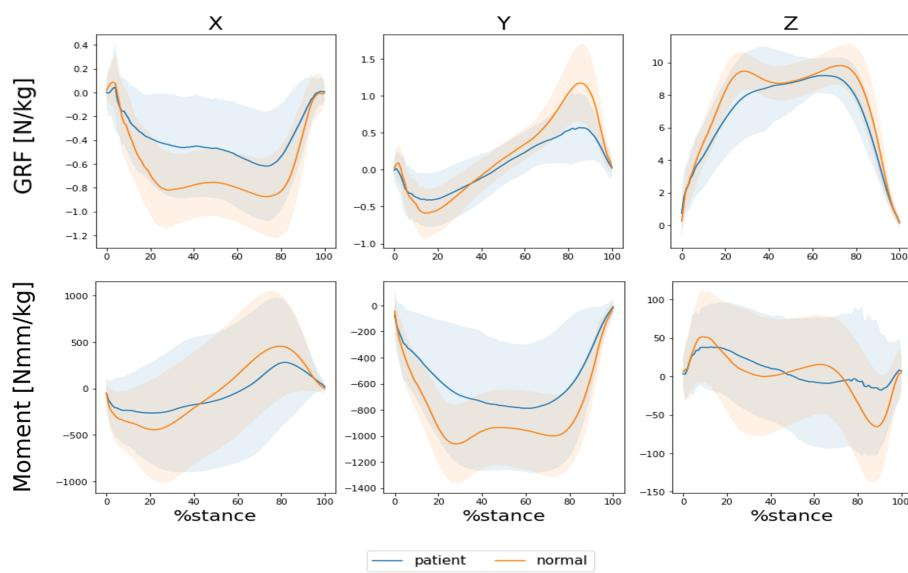
**Figure 5.** Results of measured time-series data using the force plate. Data from the stance phase in the gait cycle are measured during the one-step gait cycle, and those of the swing phase are not recorded in the experiment. The normalized time for 0~25% expresses the initial contact, 25~80% expresses the midstance, and 80~100% expresses the propulsion.
