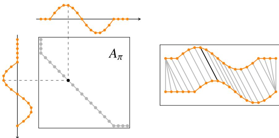
**Figure 4.** The warping path to minimize the cumulative distance between two time series is determined by the dynamic time warping (DTW) in the  $n$ -by- $m$  matrix, reproduced with permission from [14], copyright from Professor Romain Tavenard 2023. The dot on  $A_\pi$  indicates the optimal alignment of an element in  $x$  with an element in  $x'$ .
