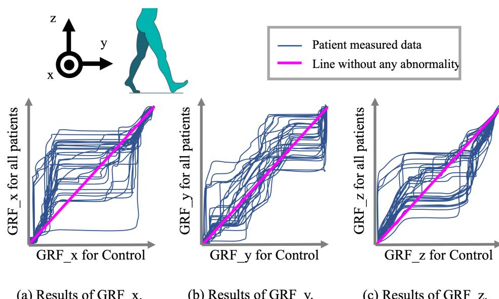
**Figure 7.** Results of accumulated cost matrices for all patients and warping path, which is expressed by dark-blue-colored curves: (a) represents the results of the x-axis ground reaction force (GRF\_x), (b) represents that of the y-axis GRF\_y, and (c) represents that of the z-axis GRF\_z.
