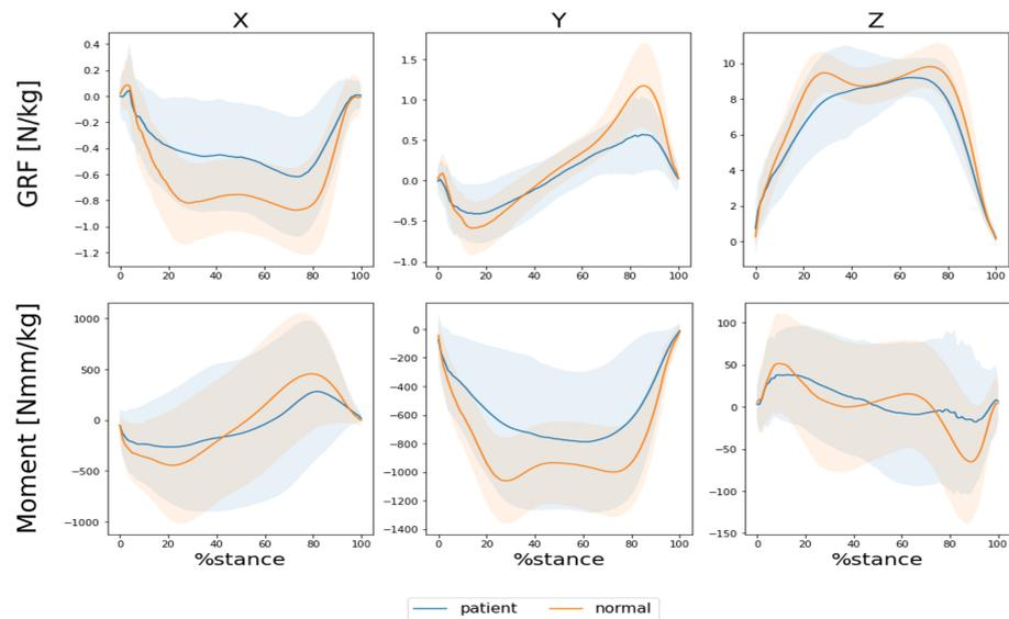
**Figure 5.** Results of measured time-series data using the force plate. Data from the stance phase in the gait cycle are measured during the one-step gait cycle, and those of the swing phase are not recorded in the experiment. The normalized time for 0~25% expresses the initial contact, 25~80% expresses the midstance, and 80~100% expresses the propulsion.
