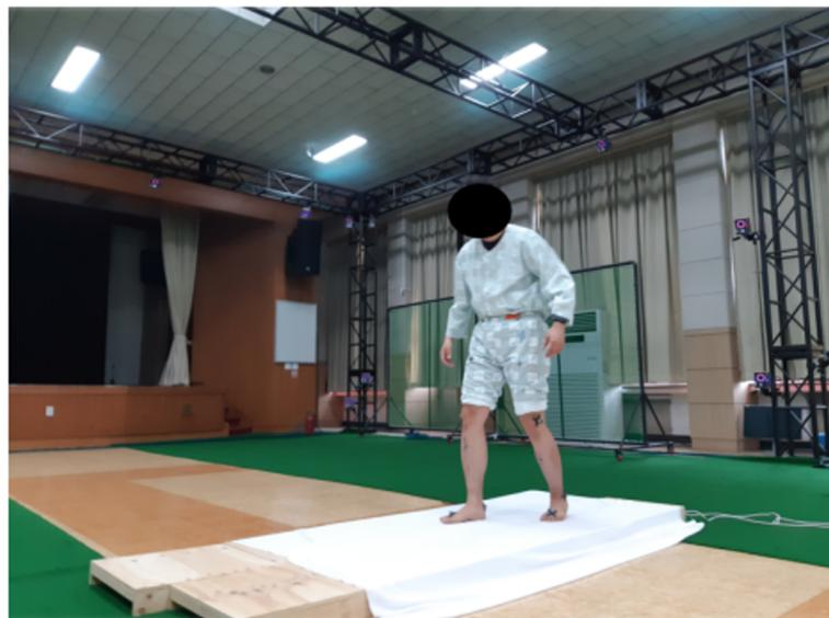
**Figure 1.** An overview of the experimental environment: Participants walk on the force plate, which can measure three directional ground reaction forces (GRFs) and moments. Because of the limitation of force plate hardware specification, the force plate allows us to measure only one-step gait in this experiment.
