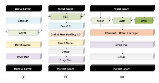
Figure 1. (a) Architecture of the CNN-LSTM model. (b) Architecture of the GRU-CNN model. (c) Architecture of the ensemble model.
