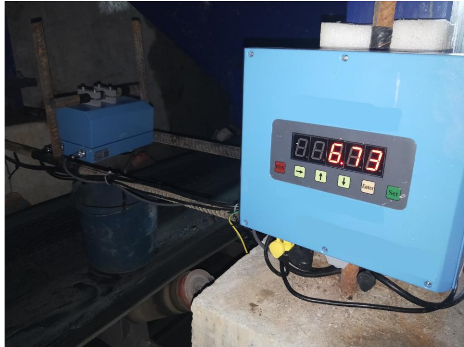
Figure 9. Testing of aggregate moisture using rapid monitoring technology.
