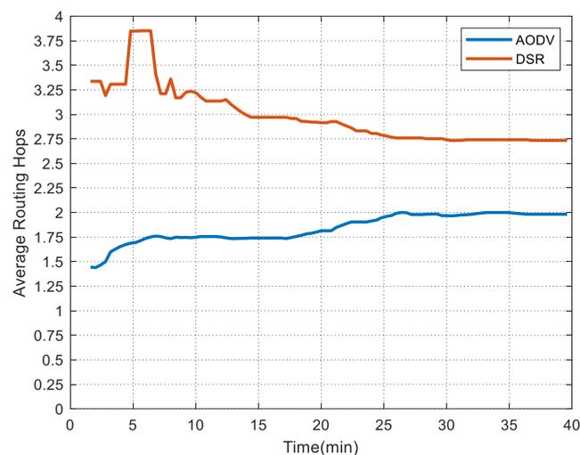
**Figure 4.** Comparison of average routing hops for AODV and DSR routing protocol.
