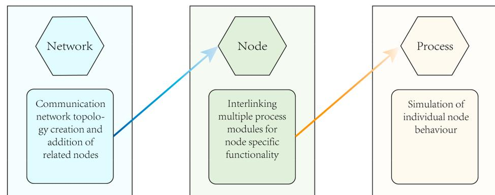
**Figure 7.** OPNET three-layer modelling mechanism.
