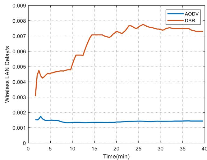
**Figure 5.** Wireless LAN delay comparison of AODV and DSR routing protocols.
