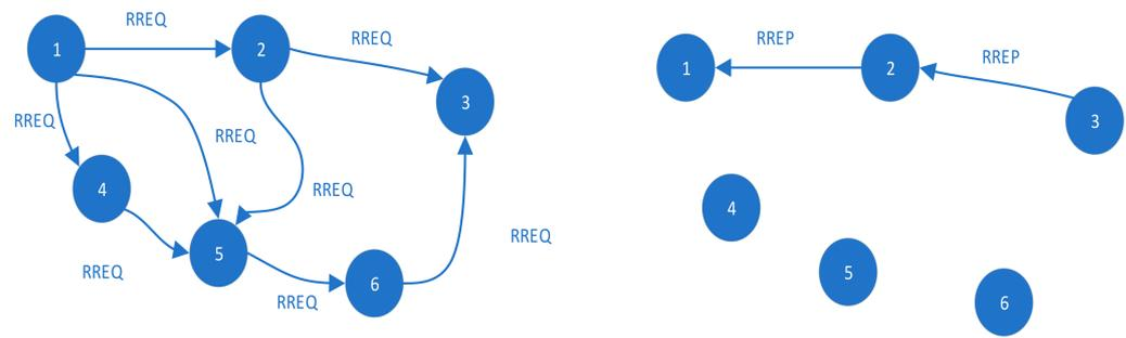
**Figure 6.** The AODV routing protocol route discovery process, where circles indicate nodes and numbers represent node indices.
