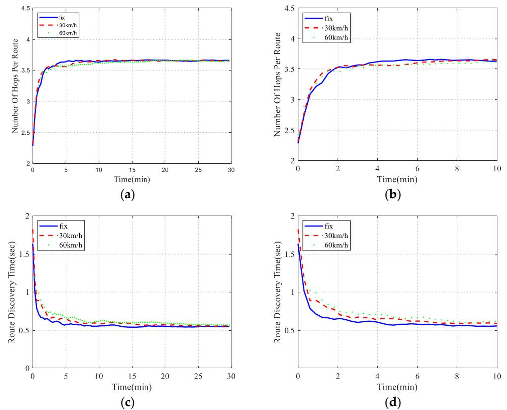
**Figure 11.** Effect of different speeds on communication stability. (a) number of hops per route, (b) local enlargement of a, (c) route discovery time, (d) local enlargement of c.
