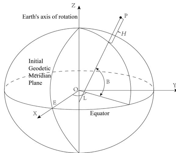
Figure 3. Geocentric coordinate system.
