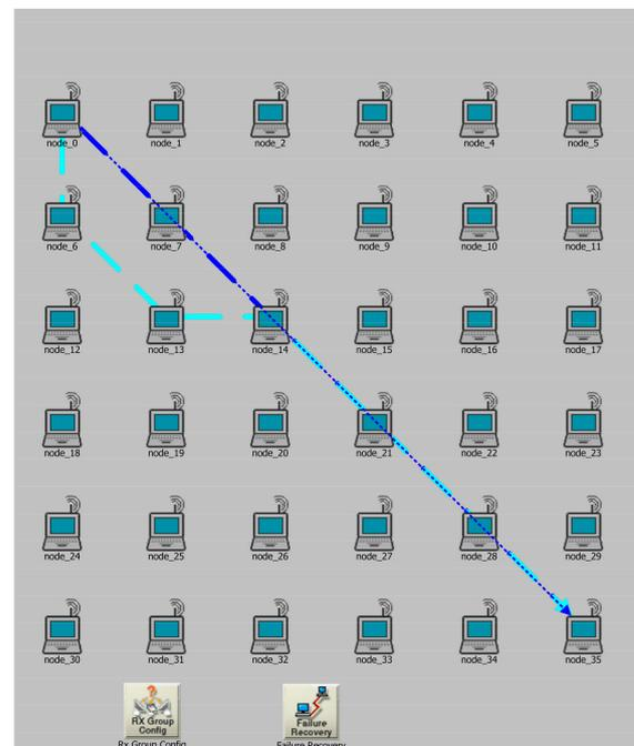
**Figure 8.** Changes in routing after *node\_7* is damaged.
