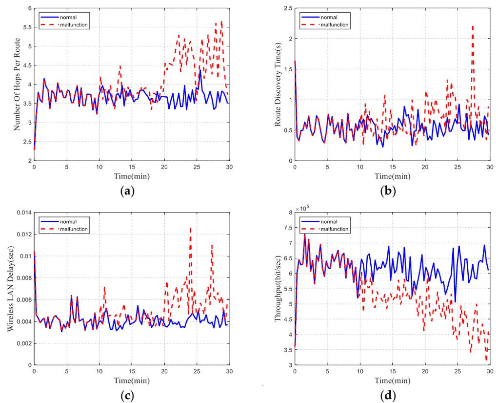
**Figure 10.** Comparative simulation data before and after node failure in terms of (a) number of hops per route, (b) route discovery time, (c) throughput, (d) wireless LAN delay.
