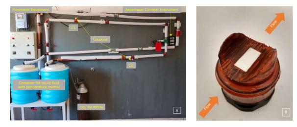
Figure 1. (A) Corrosion loop and its components; (B) coupon.
