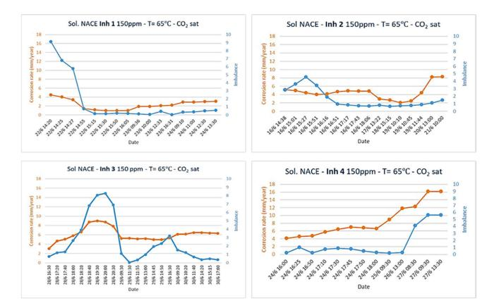
**Figure 4.** Curves obtained from each test. The *x*-axis shows the period of time, whereas the left *y*-axis shows the CR and the right *y*-axis shows the imbalance values.
