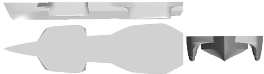
**Figure 3.** The geometry of the pentamaran.
