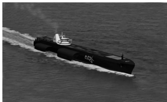
**Figure 1.** The concept design of a pentamaran [7].
