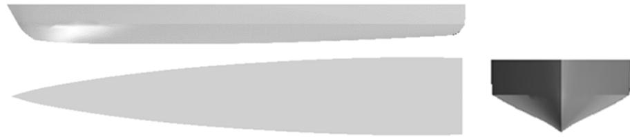
**Figure 2.** The geometry of the monohull.
