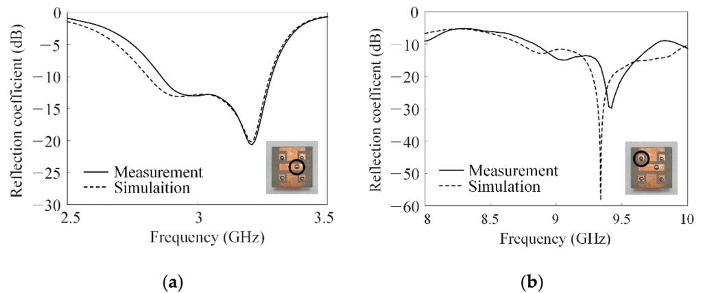
**Figure 8.** Reflection coefficients of the proposed antenna: (a) for the S-band; (b) for the X-band.
