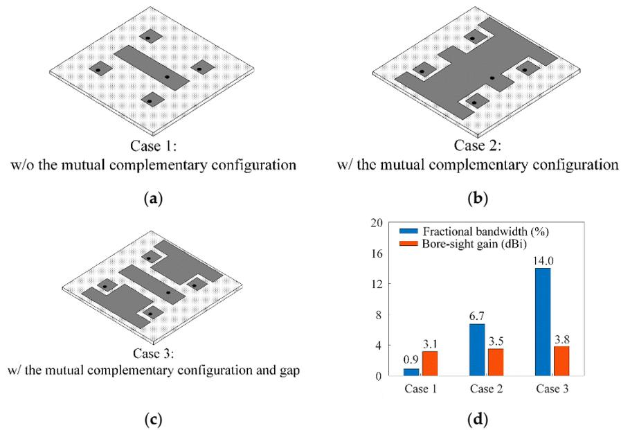
**Figure 2.** Comparison of antenna performances according to S-band element configurations: (a) without the mutual complementary configuration; (b) with the mutual complementary configuration; (c) with the mutual complementary configuration and gap; (d) bandwidths and bore-sight gains according to the S-band element configuration.
