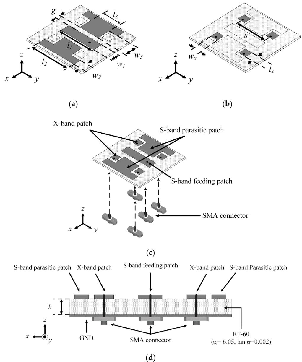
**Figure 1.** Geometry of the proposed single-layer shared-aperture antenna: (a) isometric view of the S-band element; (b) isometric view of the X-band array; (c) isometric view of the unit cell; (d) side view of the unit cell.
