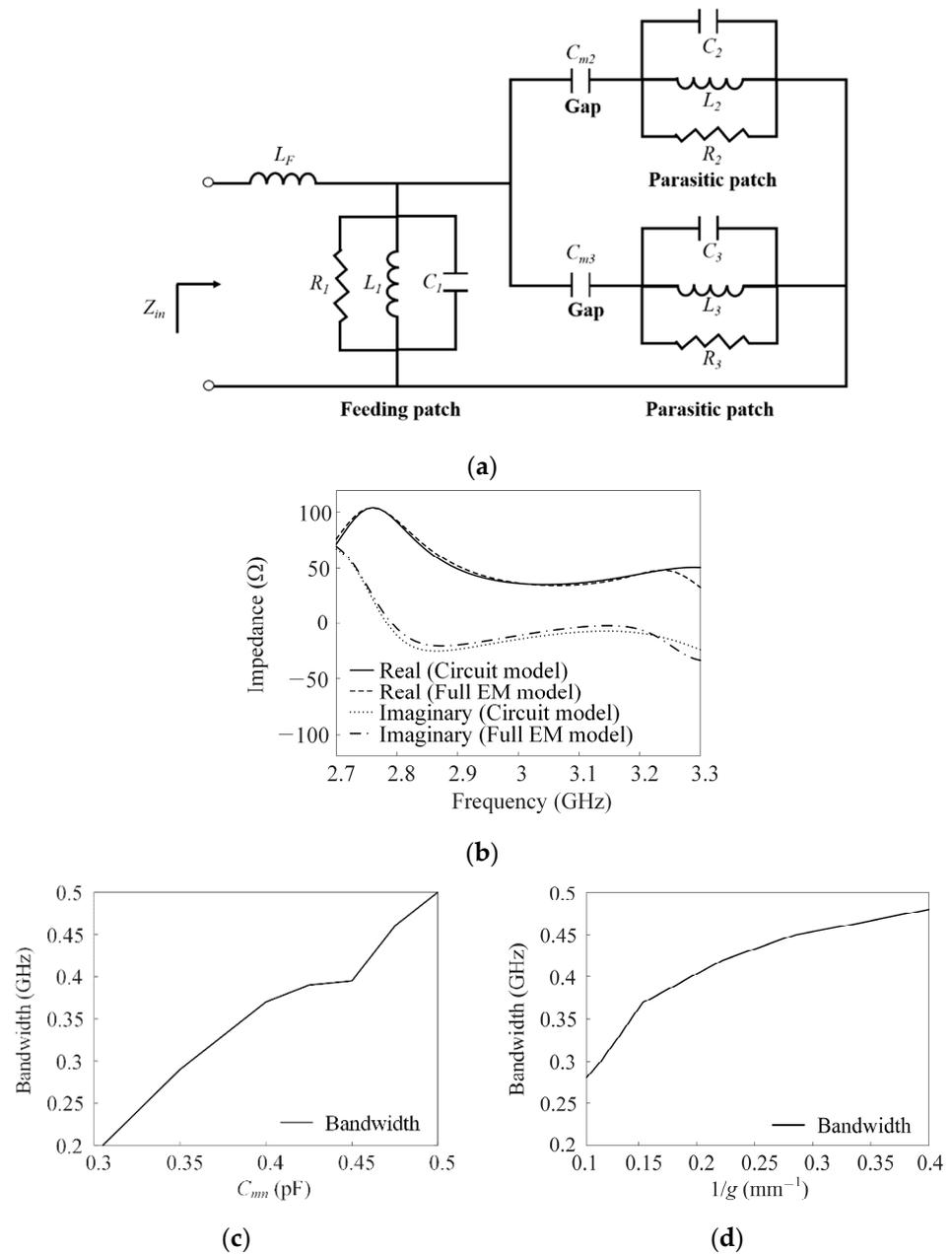
**Figure 4.** Impedance characteristics of the equivalent circuit model and the full EM simulation model: (a) equivalent circuit model; (b) comparison of impedance characteristics; (c) parametric study of  $C_{mn}$  in the equivalent circuit model; (d) parametric study of  $g$  in the full EM simulation model.
