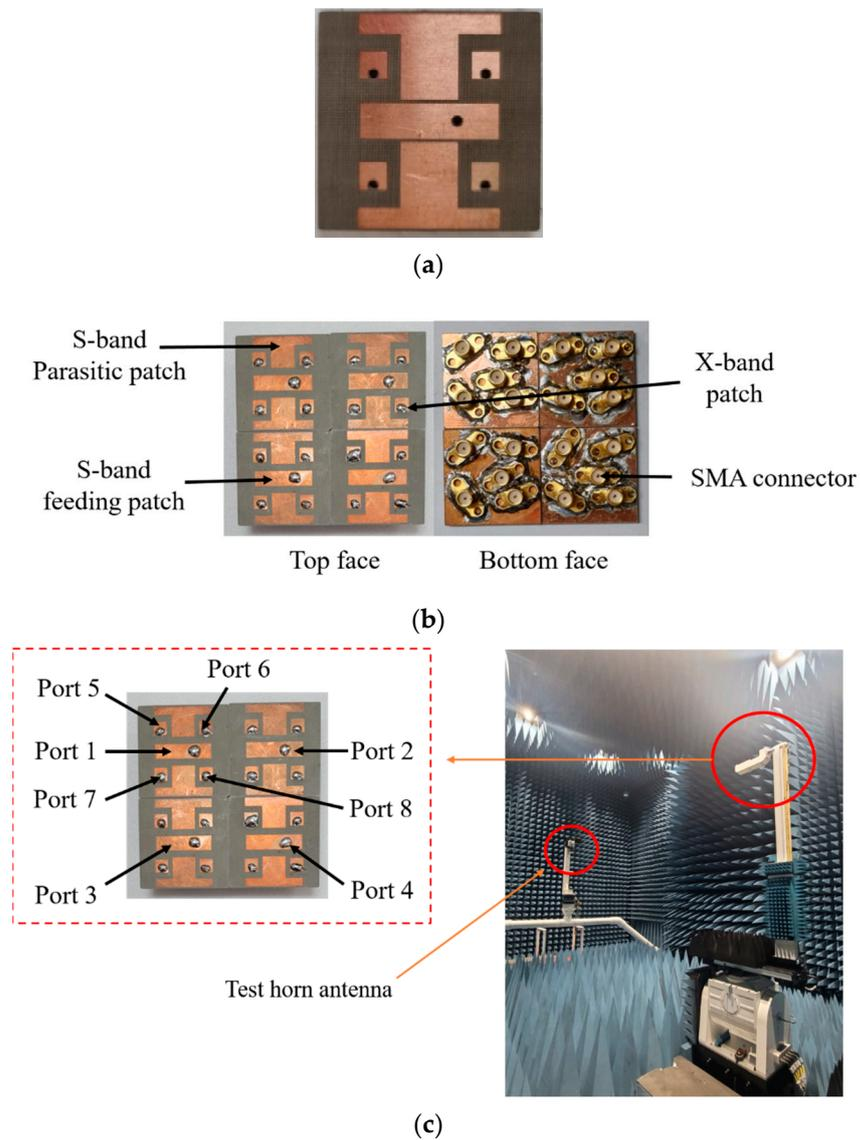
**Figure 7.** Fabricated  $2 \times 2$  array: (a) unit cell with printed radiators; (b) top and bottom faces of the  $2 \times 2$  array; (c) measurement setup.
