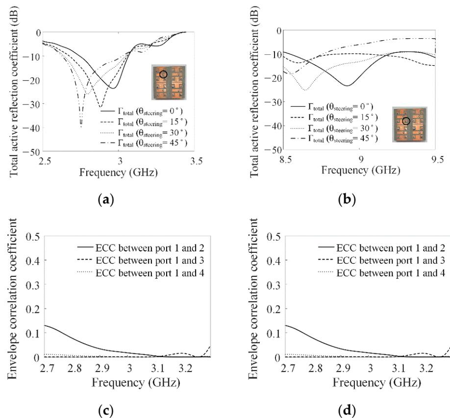
**Figure 11.** Total active reflection coefficient and envelope correlation coefficient (a) total active reflection coefficients in the S-band; (b) total active reflection coefficients in the X-band; (c) envelope correlation coefficients in the S-band; (d) envelope correlation coefficients in the X-band.
