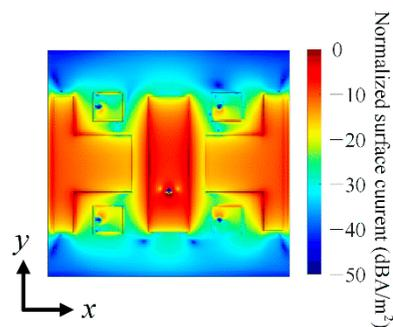
**Figure 5.** Normalized surface current distributions of the S-band element.
