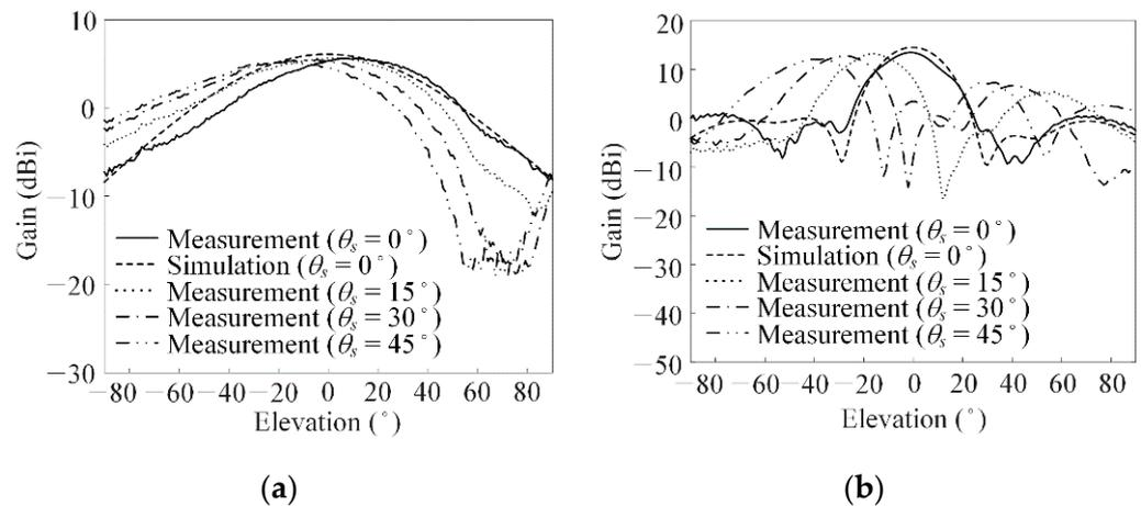
Figure 10. Beam-steering characteristics of the proposed antenna: (a) S-band; (b) X-band.
