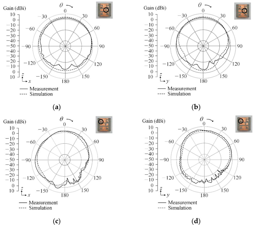
**Figure 9.** 2D radiation patterns of the proposed antenna: (a) S-band element in the  $zx$ -plane; (b) S-band element in the  $zy$ -plane; (c) X-band element in the  $zx$ -plane; (d) X-band element in the  $zy$ -plane.
