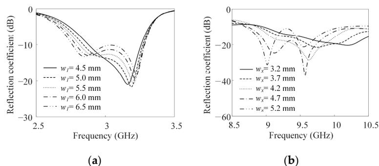
**Figure 3.** Reflection coefficient according to patch widths: (a) for the S-band element; (b) for the X-band elements.
