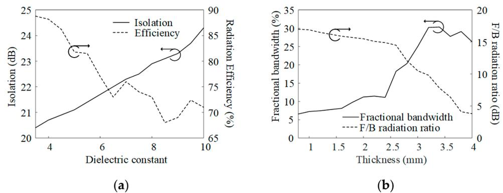
**Figure 6.** Antenna performance variations of the X-band element according to the dielectric constant and the thickness of the substrate: (a) isolation and radiation efficiency according to the dielectric constant; (b) bandwidth and front-to-back (F/B) radiation ratio according to substrate thickness.
