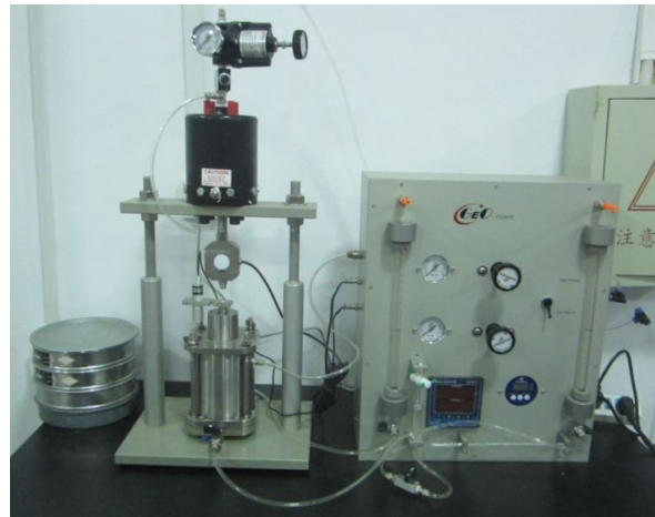
Figure 5. Test system of the soil–water characteristic curve using the pressure plate apparatus.
