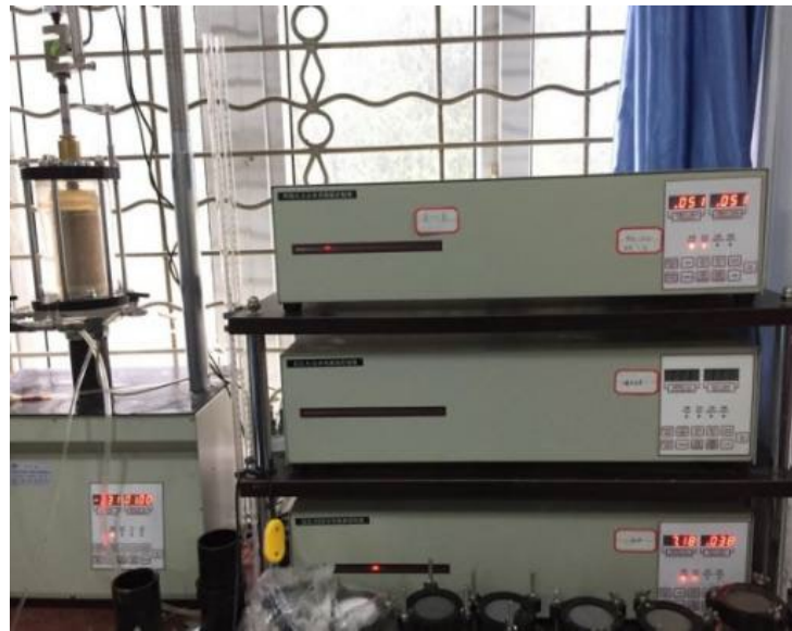
Figure 7. Test system of the triaxial shear apparatus.
