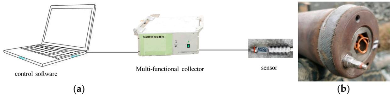
**Figure 4.** Pressure test system: (a) composition and connection mode of pressure test system; (b) installation of sensors.
