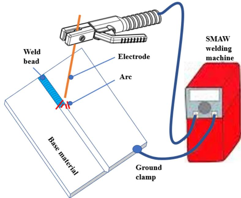
Figure 2. Mechanism of SMAW welding process.
