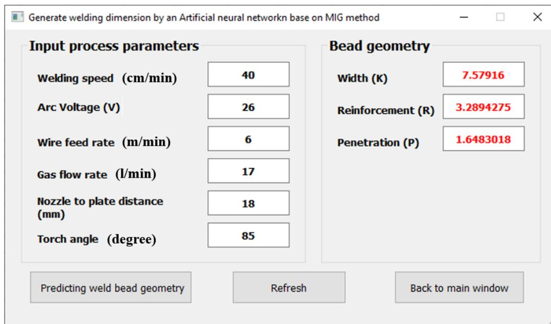
Figure 11. Screenshot of the MIG welding module of the developed predictive system.
