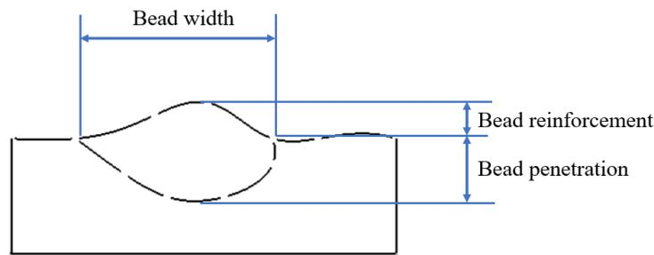
Figure 5. Geometry of weld bead.
