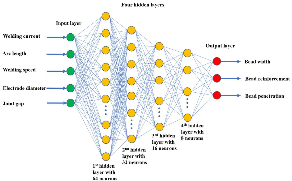
Figure 7. Deep learning neural network architecture for the SMAW welding process.
