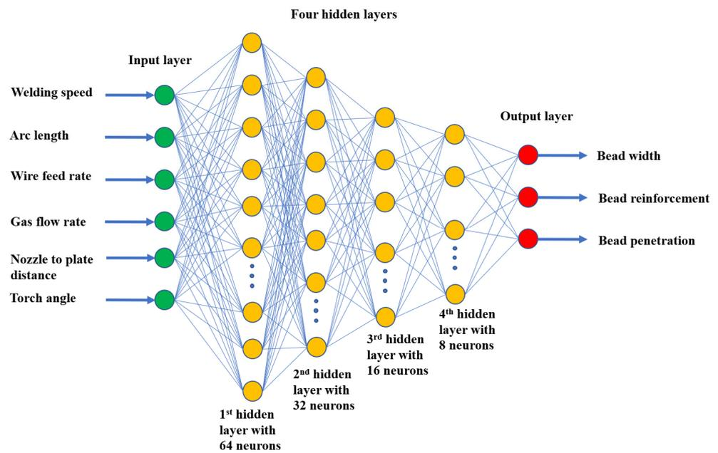
Figure 8. Deep learning neural network architecture for the MIG welding process.
