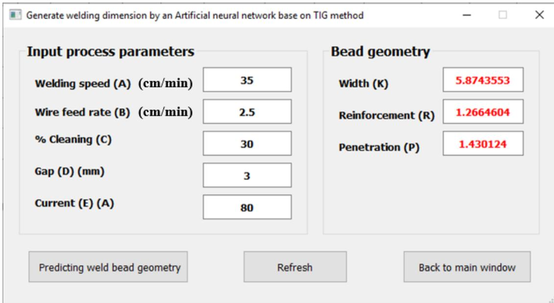
Figure 10. Screenshot of the TIG welding module of the developed predictive system.
