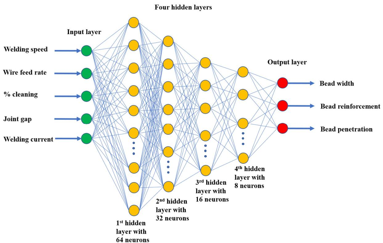
**Figure 6.** Deep learning neural network architecture for the TIG welding process.
