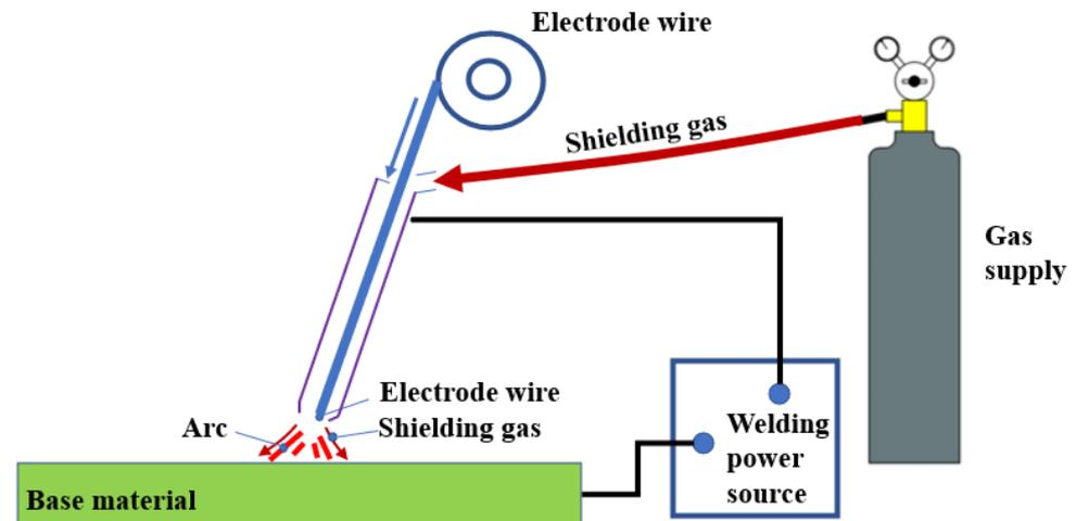
**Figure 4.** Mechanism of MIG welding process.
