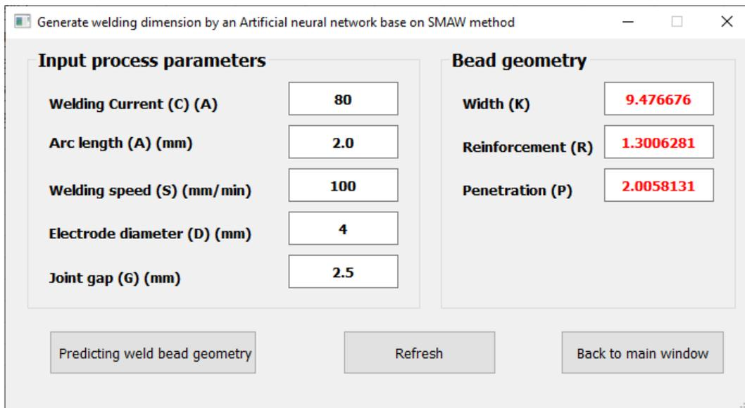
Figure 12. Screenshot of the SMAW welding module of the developed predictive system.
