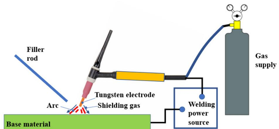
Figure 3. Mechanism of TIG welding process.
