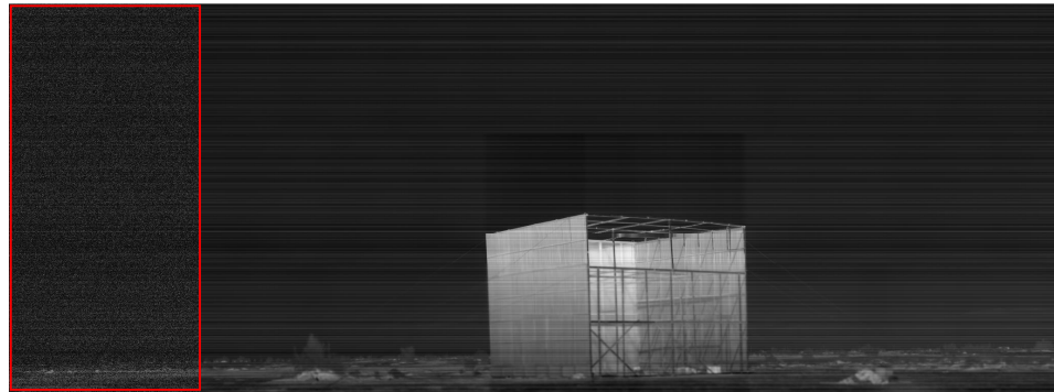
Figure 4. Infrared scan image with the addition of Gaussian noise. Due to the very high resolution of the infrared column scan image ( 3053 \times 55,000 ), only a portion of the scanned image ( 3053 \times 8192 ) is displayed in this figure. The image within the red border is the image utilized for the linear fitting model in Section 2.1, with a resolution of 3053 \times 1500 pixels.
