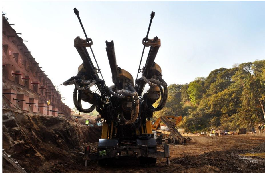
**Figure 3.** Jumbo with three drilling arms.
