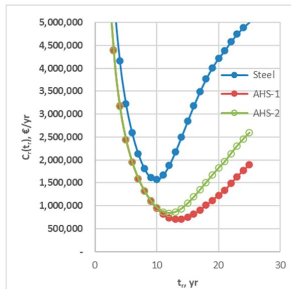
Figure 10. Total cost of repair per unit of time.
