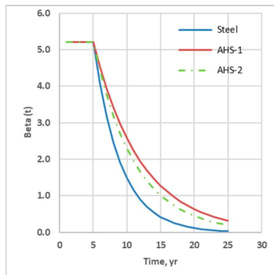
**Figure 3.** Beta-reliability index as a function of corrosion degradation (without repair and maintenance).
