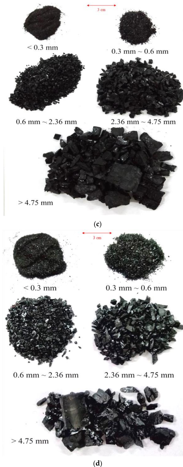
Figure 7. Failure morphology of coal specimens under differential dynamic impact velocities after sieving. (a) v = 2.675 \text{ m}\cdot\text{s}^{-1} . (b) v = 3.275 \text{ m}\cdot\text{s}^{-1} . (c) v = 4.024 \text{ m}\cdot\text{s}^{-1} . (d) v = 5.011 \text{ m}\cdot\text{s}^{-1} .
