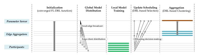
Figure 10. eFL procedures for the aggregation for the averaged global model.
