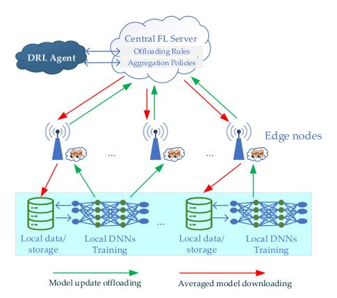
**Figure 9.** Embedded DRL-based optimization engine for offloading rules and aggregation policies in the central FL server.
