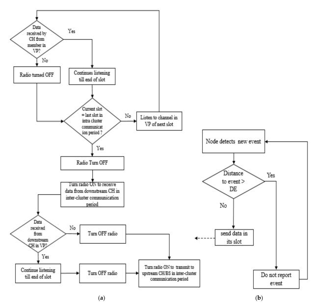
**Figure 5.** Steady-State Phase in Proposed Model: (a) Functioning of CH and (b) Functioning of member node.
