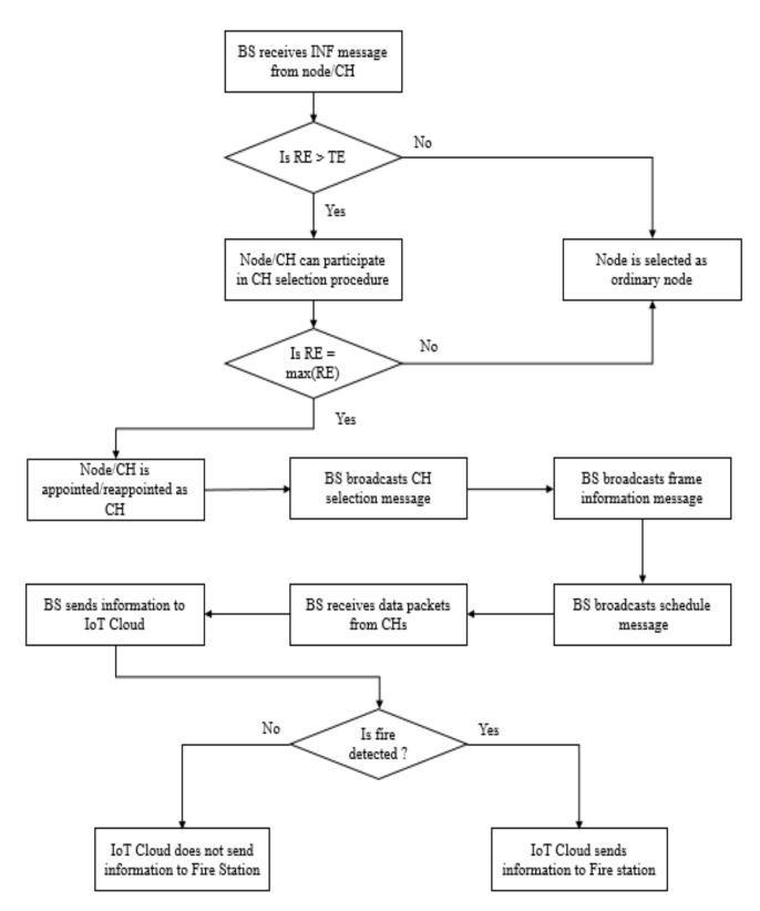
Figure 6. Functioning of the BS in a complete round.
