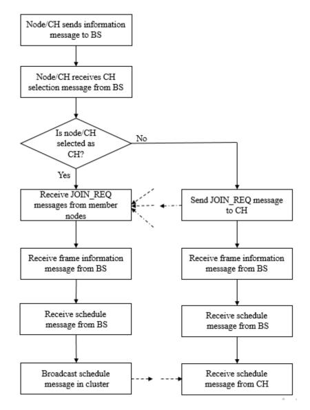
Figure 3. Setup Phase in Proposed Model.
