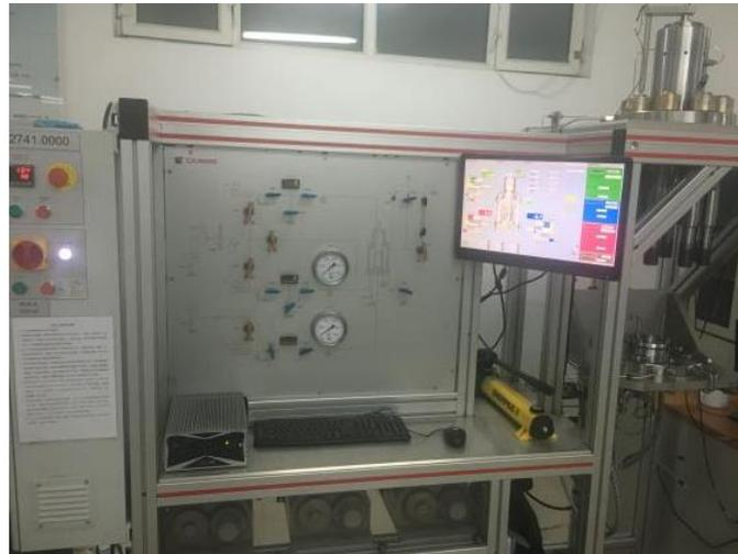
**Figure 1.** TOP INDUSTRIE Rock 600-50 Rock automatic servo rheometer.
