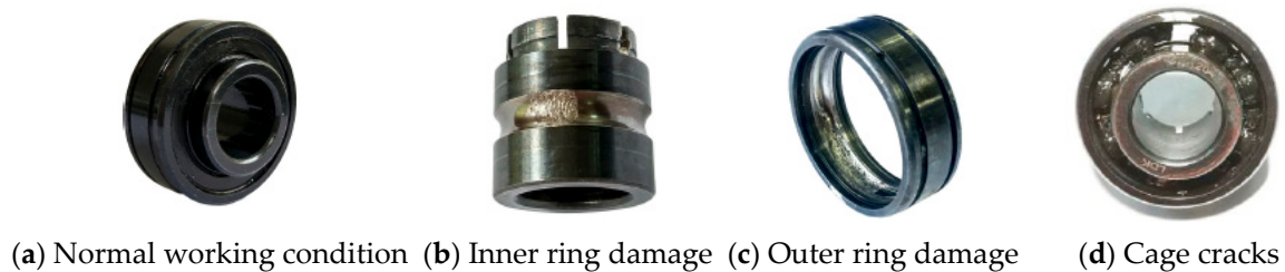
Figure 6. Images of typical bearing failure types.
