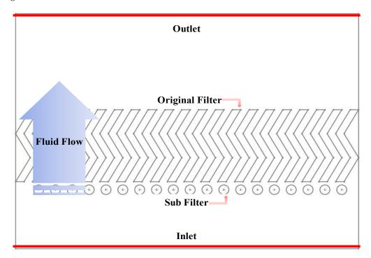
Figure 6. Analytical boundary conditions for sub-filters mounted under the filter.
