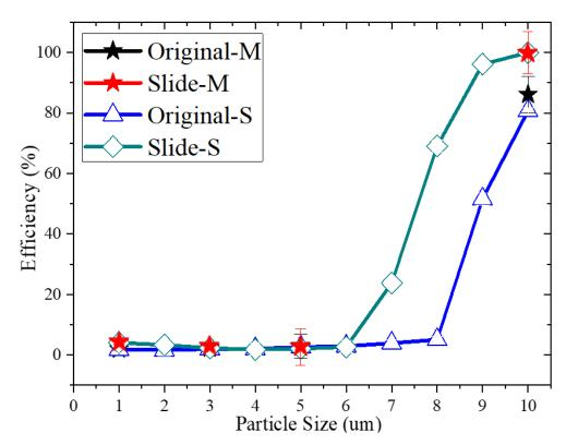
Figure 13. Comparison graph of filter with Coanda effect applied.
