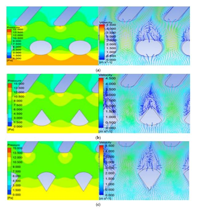
Figure 8. (a) Circle; (b) Droplet; and (c) Cone pressure and vector contours.
