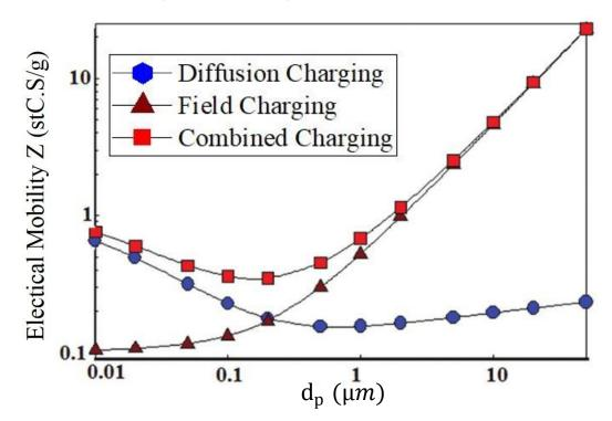
Figure 15. The combined charging is a function of the particle diameters.
