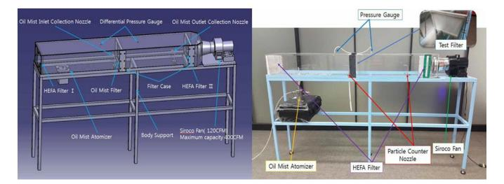
Figure 11. Design drawing and filter experiment device.
