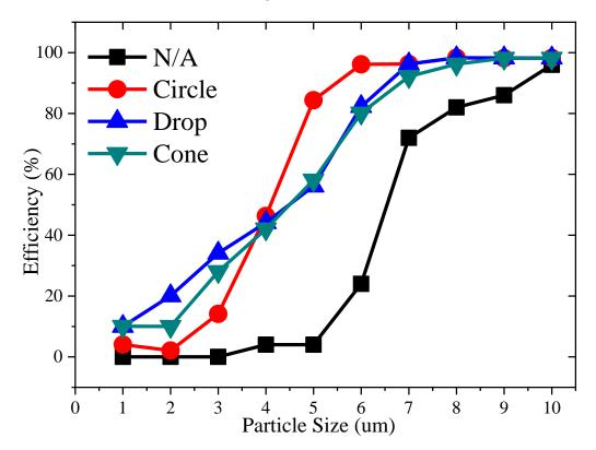
Figure 9. Efficiency by particle size with sub-filter applied.
