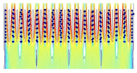
Figure 17. Particle tracking contour of I-filter.
