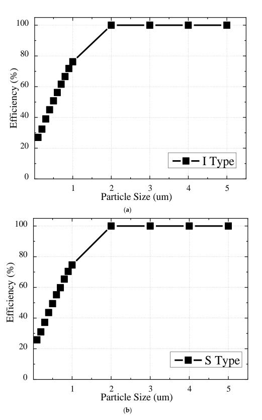
Figure 18. Efficiency comparison of I-Filter (a) and S-Filter (b).
