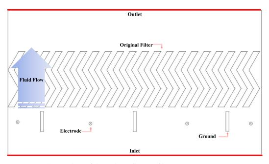
Figure 16. Boundary condition of electric dust-collection S-filter.
