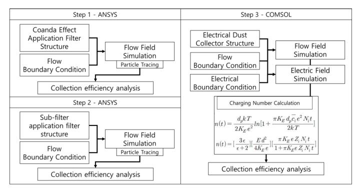
Figure 1. Physical and electrical filter simulation flow.
