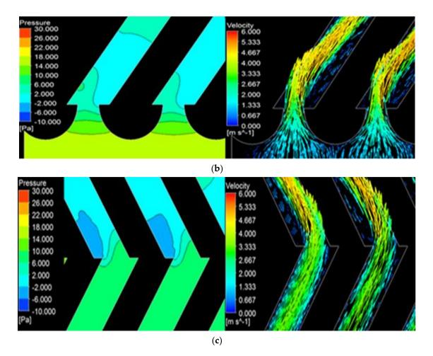
Figure 4. (a) Original; (b) Bottom; and (c) Slide model pressure and vector contours.
