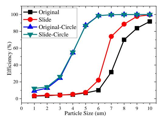
Figure 10. A comparison graph of filters with and without sub-filters.
