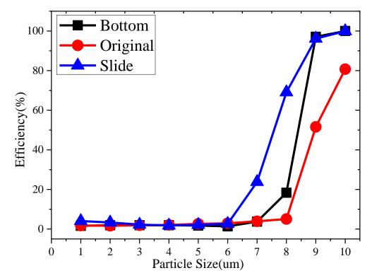
Figure 5. Efficiency by particle size in Coanda-applied filter.
