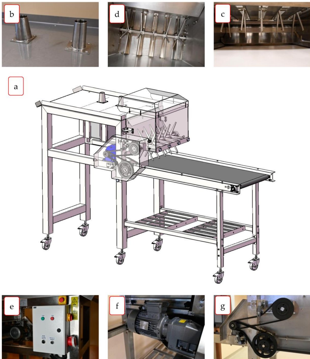
Figure 4. Prototype of the designed vegetable crusher: (a) general view; (b) floretting knives; (c) crushing chamber; (d) screen at the bottom of the crushing chamber; (e) power control box, (f) electric motor; and (g) V-belts.
