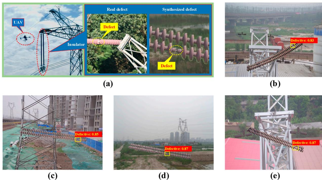
**Figure 10.** An example of the detection of defective insulators using our model: (a) the schematic of the insulator defect detection and its images; (b–e) the identification effect of different defective insulators synthesized with ground-truth images.
