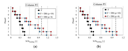
**Figure 15.** Buckling checks in the most stressed columns in the eight-story MRF: (**a**) column P2 and (**b**) column P5.
