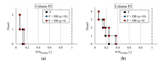
Figure 14. Buckling checks in the most stressed column in (a) two-story MRF and (b) four-story MRF.
