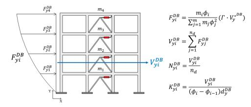
**Figure 9.** Graphical representation of the procedure for distributing the properties of the damped braces at the stories of the frame.
