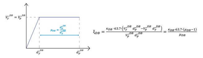
**Figure 7.** Force-displacement of the equivalent SDOF damped brace.  $V_y^{*DB}$  and  $V_p^{*DB}$ : yield and ultimate force;  $d_y^{*DB}$  and  $d_p^{*DB}$ : yield and ultimate displacement;  $\mu_{DB}$ : ductility factor.
