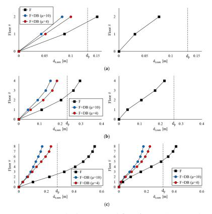
**Figure 12.** Maximum displacement at each floor of case-study MRFs with and w/o damped braces: (a) two-story, (b) four-story, and (c) eight-story structures.
