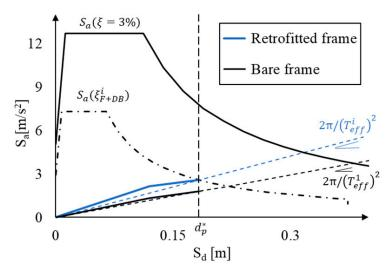
**Figure 8.** Graphical representation of the iteration of Step 4 for evaluating the properties of the equivalent SDOF damped brace.
