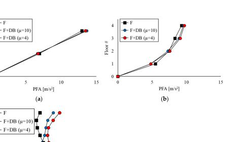
Figure 13. Peak Floor Acceleration of the case-study MRFs with and w/o damped braces: (a) twostory, (b) four-story, and (c) eight-story structures.
