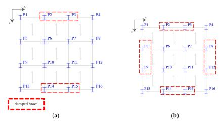
**Figure 10.** Plan layout of damped braces in (**a**) two-story and four-story structures, (**b**) eight-story structure.
