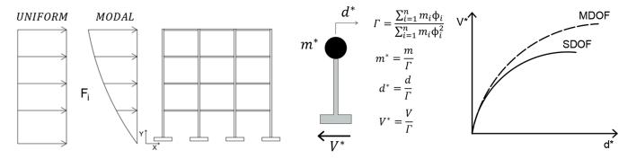
Figure 3. Determination of main frame capacity curves according to IBC.
