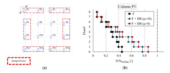
**Figure 16.** (**a**) new plan layout of damped braces in the eight-story MRF; (**b**) buckling checks in column P3 of the retrofitted frame.
