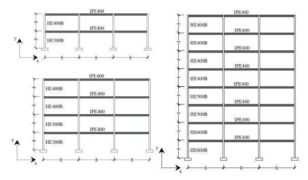
Figure 2. Elevation views of case-study structures (dimensions in m).
