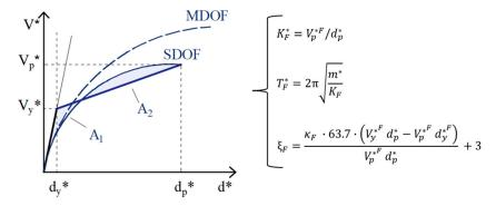
**Figure 5.** Determination of the equivalent bilinear curve of the main frame according to the Commentary of IBC.
