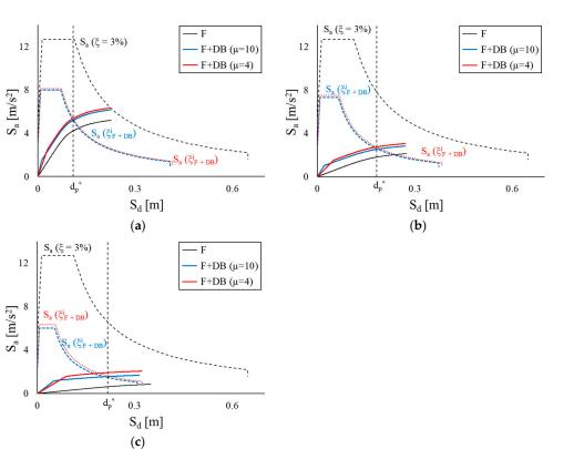
Figure 11. Results of NSLAs in X-direction of (a) two-story, (b) four-story, and (c) eight-story structures.
