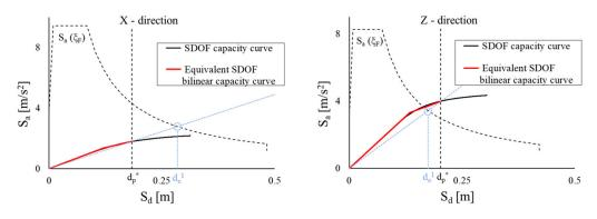
**Figure 6.** Comparison of the equivalent SDOF bilinear capacity curves of the four-story frame with the relevant demand response spectra in X- and Z-directions.
