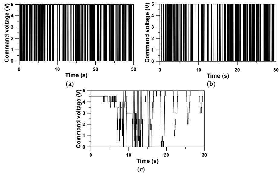
Figure 18. Time histories of command voltage (EV1): (a) groundhook algorithm, (b) skyhook algorithm, (c) DQN algorithm.
