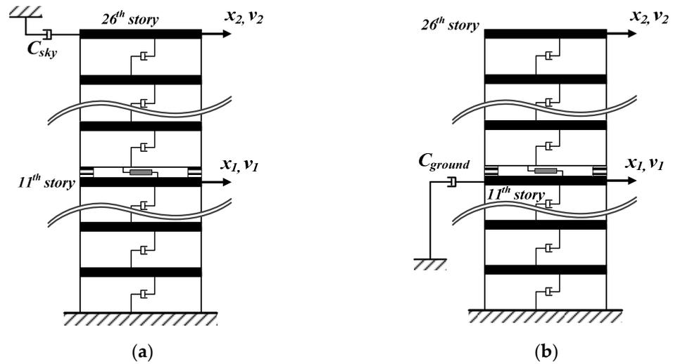
Figure 12. Idealized semi-active control configurations: (a) skyhook, (b) groundhook.
