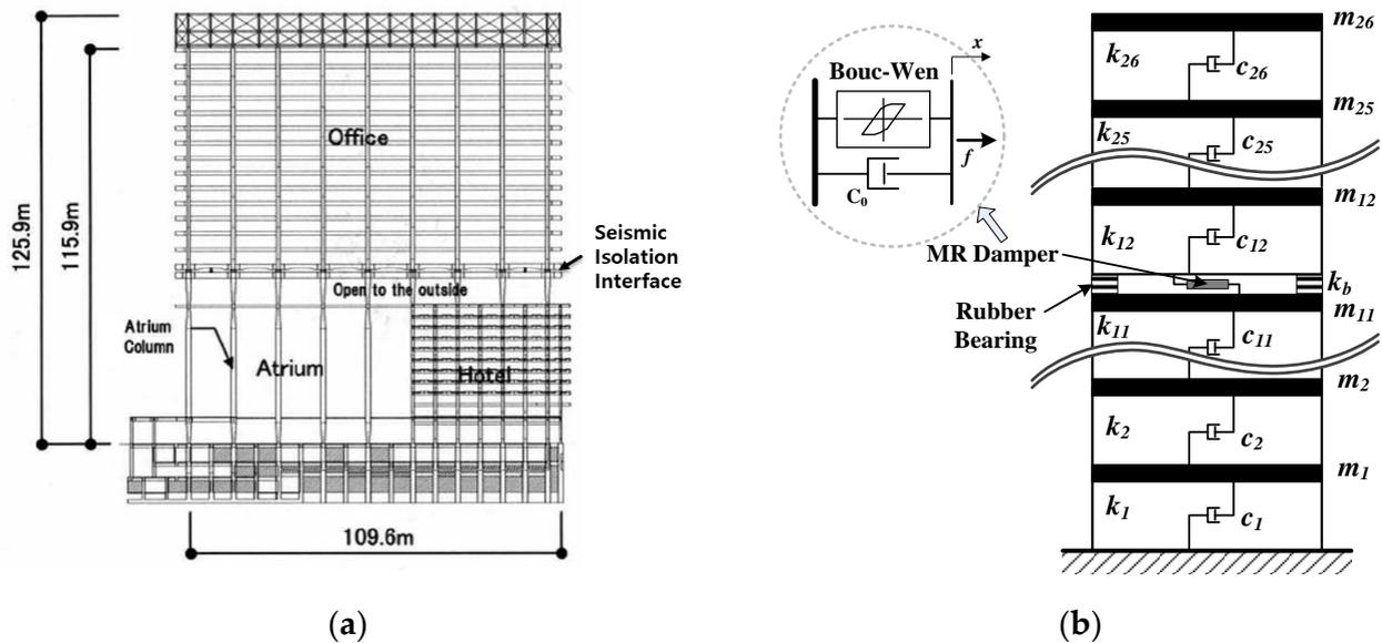
Figure 5. Sample building structure with a mid-story isolation system: (a) elevation of the Shiodome Sumitomo building [20], (b) analytical model with SMIS.
