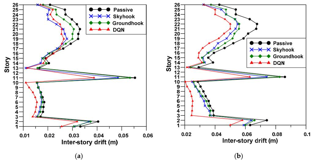
Figure 17. Peak inter-story drift of each control algorithm: (a) responses to EV1, (b) responses to EV2.
