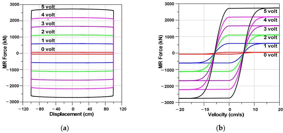
**Figure 6.** Hysteresis loops of the MR damper: (a) displacement—force hysteresis loop, (b) velocity—force hysteresis loop.
