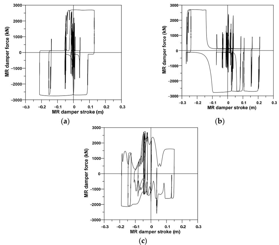
**Figure 19.** MR damper stroke-and-force relationship (EV1): (a) groundhook algorithm, (b) skyhook algorithm, (c) DQN algorithm.
