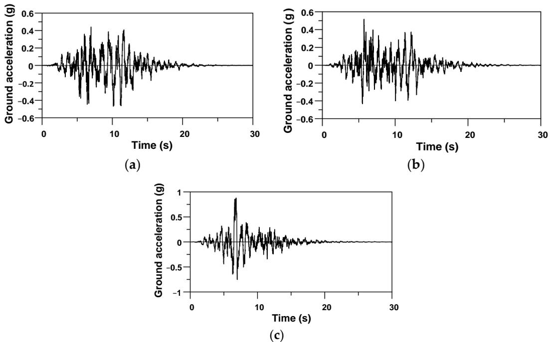
**Figure 7.** Time histories of artificial ground acceleration. (a) Earthquake for training. (b) Earthquake for verification1 (EV1). (c) Earthquake for verification2 (EV2).
