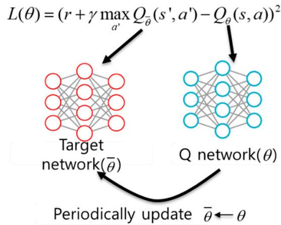
Figure 4. Target network separation.
