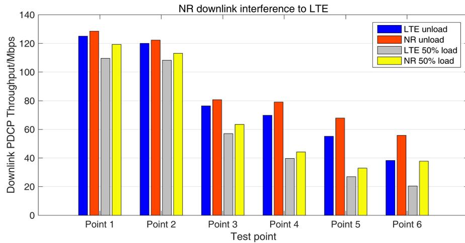
Figure 15. NR to LTE downlink interference test results.
