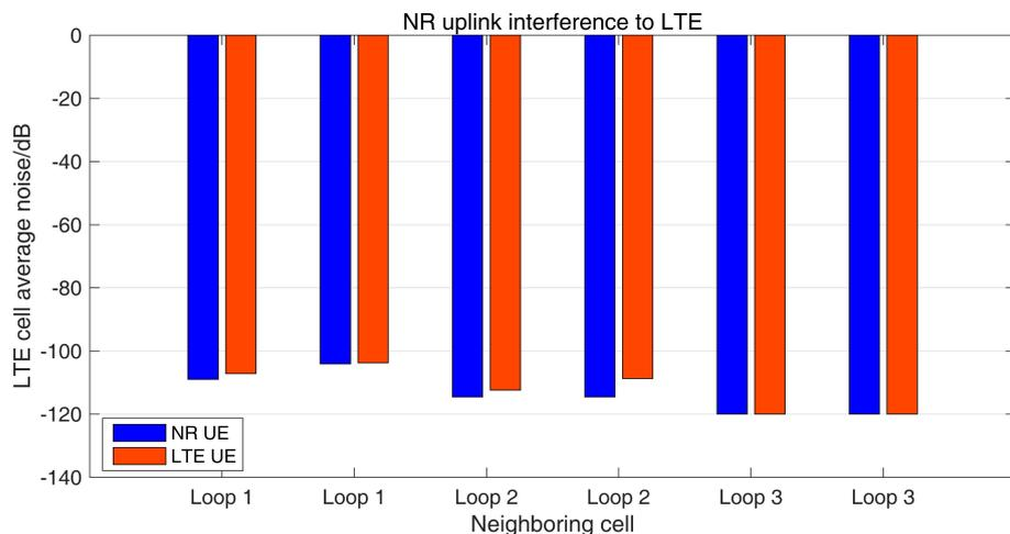
Figure 16. NR terminal to LTE uplink interference test results.
