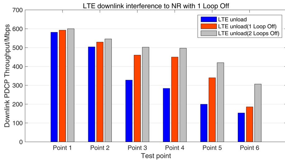
Figure 18. LTE to NR downlink interference test results—buffer setting (no load).
