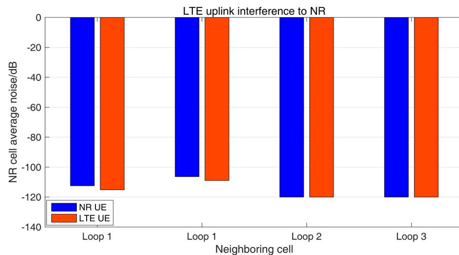
**Figure 17.** LTE terminal to NR uplink interference test results.
