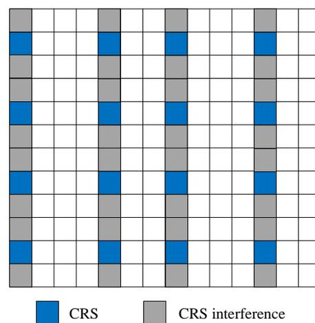
**Figure 6.** Schematic diagram of DSS interference.
