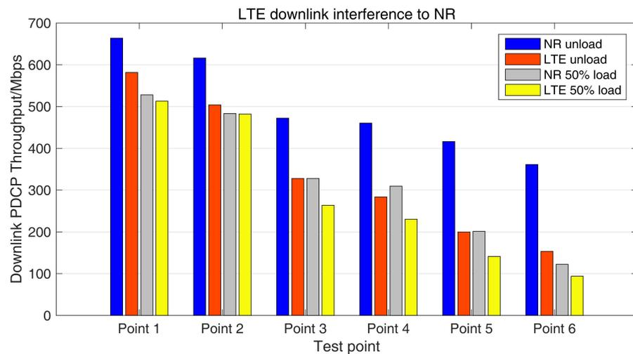
**Figure 14.** LTE to NR downlink interference test results.
