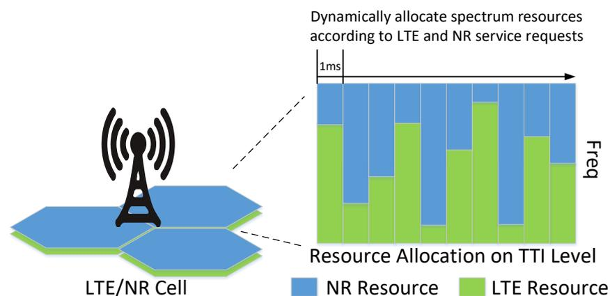
Figure 2. DSS dynamically adjusts spectrum resources.
