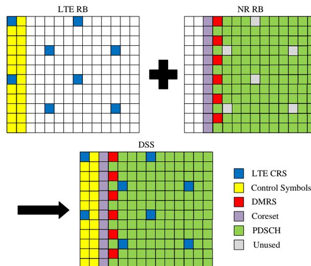
Figure 9. Schematic diagram of rate matching.
