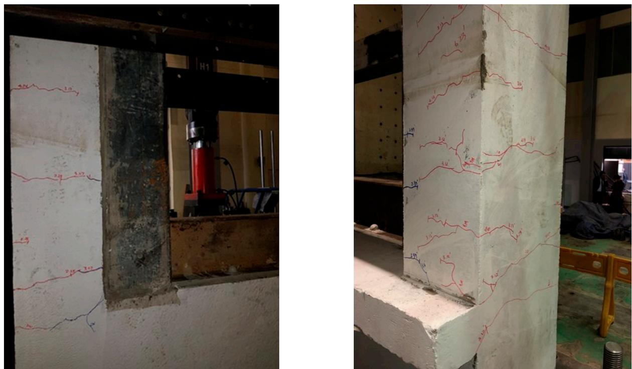
Figure 12. Test results of the PD-CCSS specimen (300 cm/s<sup>2</sup>, final).
