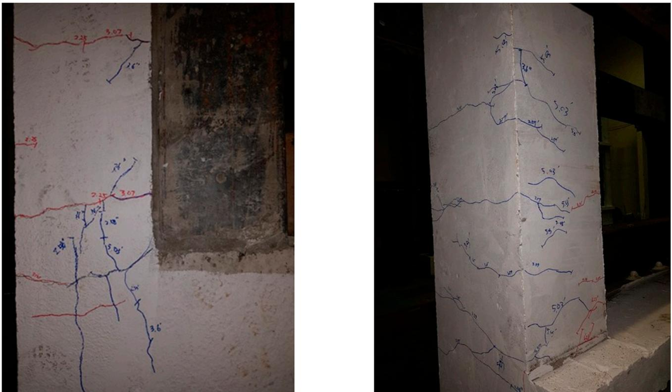
Figure 13. Test results of the PD-CCSS specimen ( $400 \text{ cm/s}^2$ , final).
