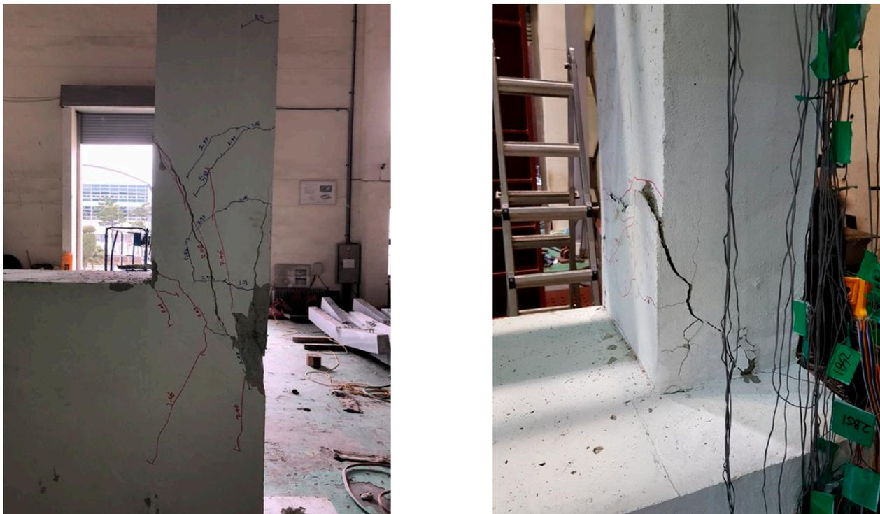
**Figure 10.** Test result of PD-FR specimen (200 cm/s<sup>2</sup>, final).
