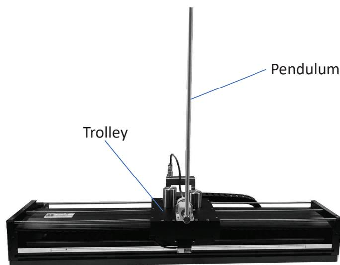
Figure 1. Inverted pendulum system diagram.
