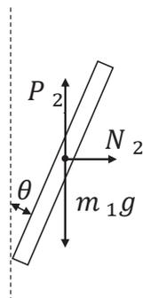
Figure 4. Force analysis of the pendulum.
