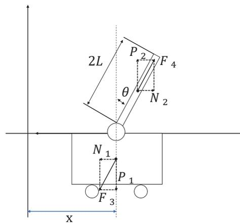
Figure 2. First-order inverted pendulum physical model.
