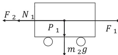
Figure 3. Force analysis of the trolley.
