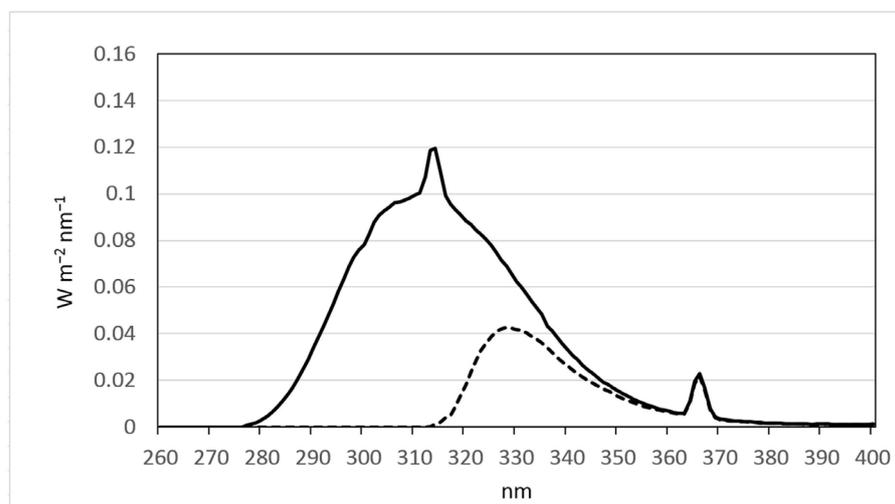
**Figure 1.** Spectral irradiance of Q-Panel UVB 313 fluorescent lamps, unfiltered (solid line) and filtered with polyester film (dotted line). The intensity of the lamps was the same as that used for the experiment.
