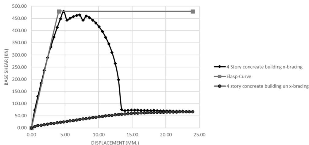
**Figure 8.** Comparison between masonry wall building with x-bracing and original wall building without x-bracing concrete frame.
