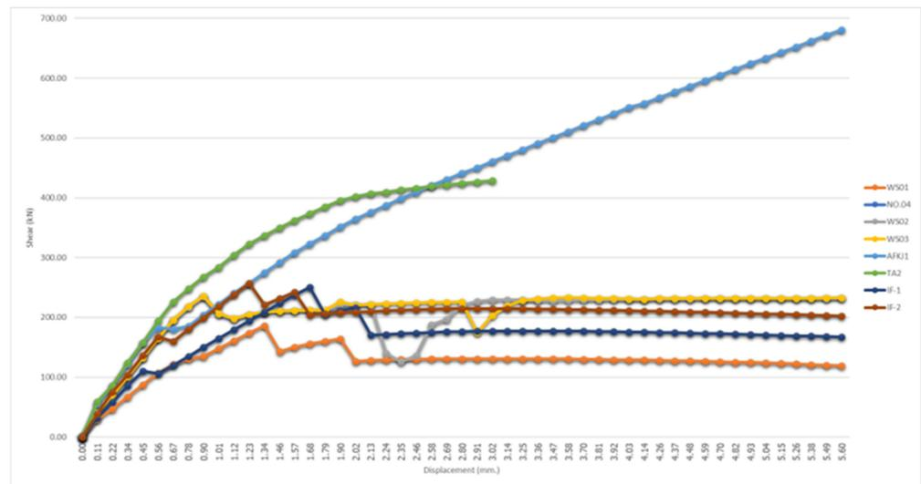
Figure 3. Relationship between the lateral force and lateral displacement of the model samples.
