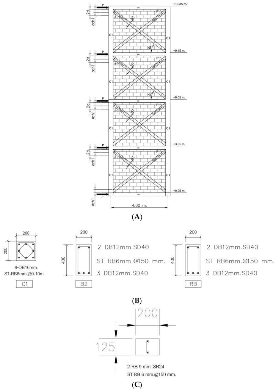
**Figure 6.** Masonry walls, columns, and beams reinforced with x-bracing concrete frame. (A) Single-span reinforced building frame; (B) cross-section of the reinforced column and beam; (C) cross-section of the reinforced x-bracing concrete frame.
