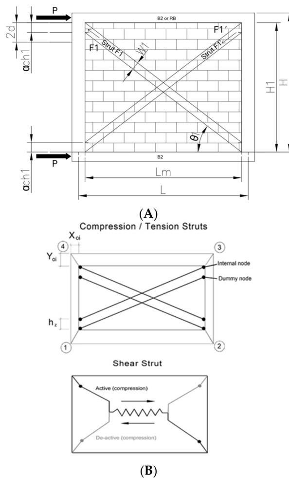
**Figure 1.** Model of masonry wall building reinforced with x-bracing frame. (A) Model of masonry wall building reinforced with x-bracing concrete frames for compressive strength. (B) Model of masonry wall building reinforced with x-bracing concrete frame for compression/tension and shear strut.
