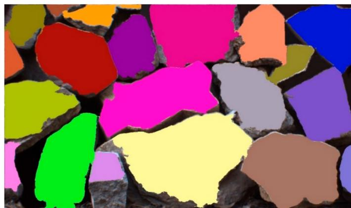
**Figure 5.** Segmentation results of the ore rock image.
