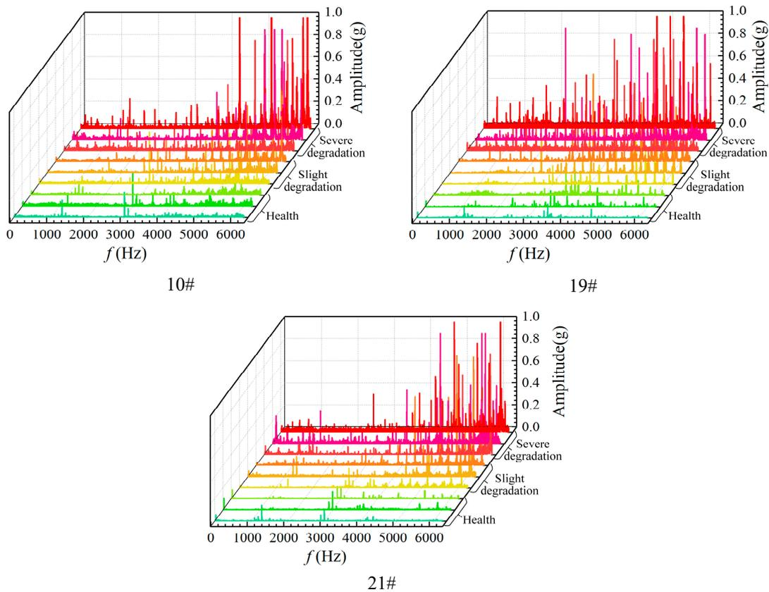
Figure 14. Comparison of spectral maps at different degradation stages.
