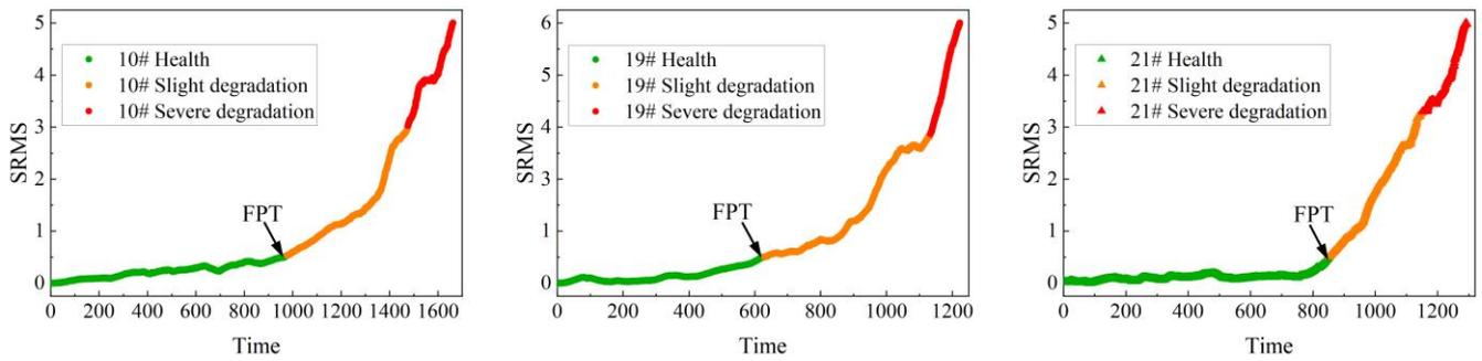
Figure 12. The degradation stage division results for three datasets.
