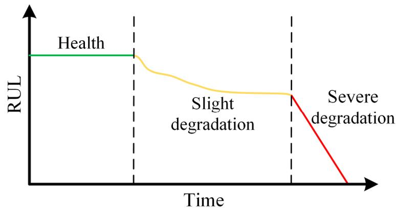
Figure 8. The degradation stage of WT bearings.
