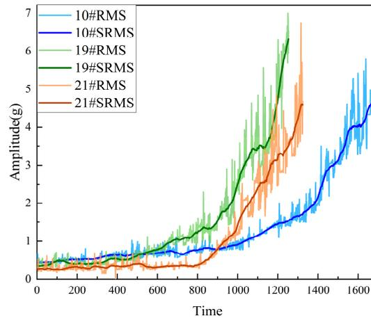
Figure 11. SRMS curve of three WTs after SG filtering.
