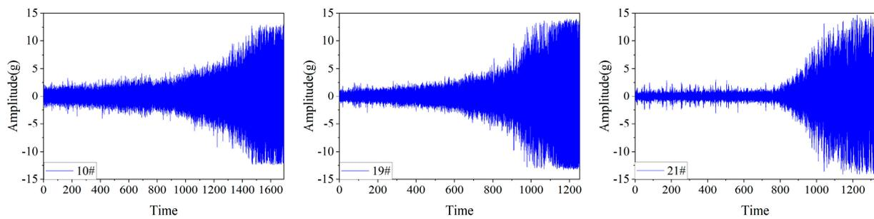
Figure 3. Time domain diagram of WT generator bearings.
