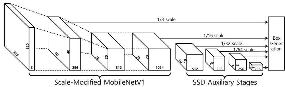
Figure 1. MobileNet V1 and SSD with input image 320 × 320.
