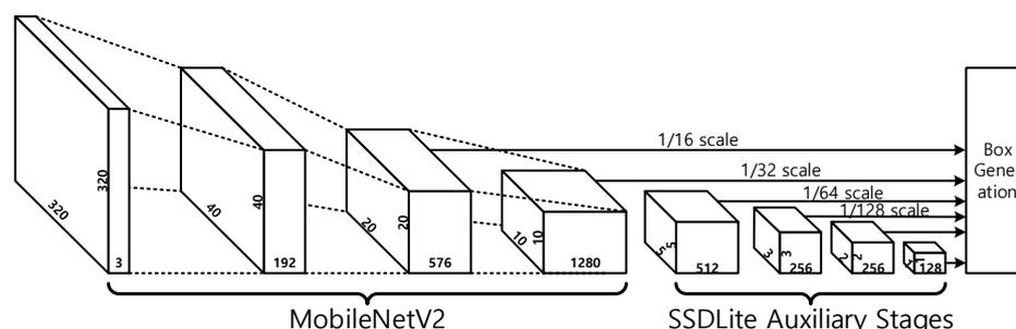
Figure 2. MobileNet V2 and SSDLite with input image 320 × 320.
