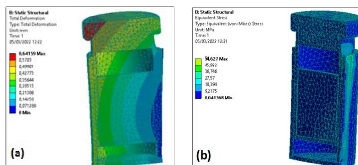
**Figure 9.** (a) Deformation and (b) Von Mises stress under distributed force (Reproduced from [24] with permission from Springer Nature Switzerland AG).
