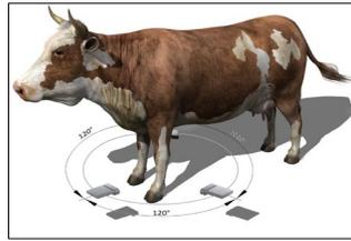
**Figure 2.** Acquisition layout using three Microsoft Kinect DK scanners.
