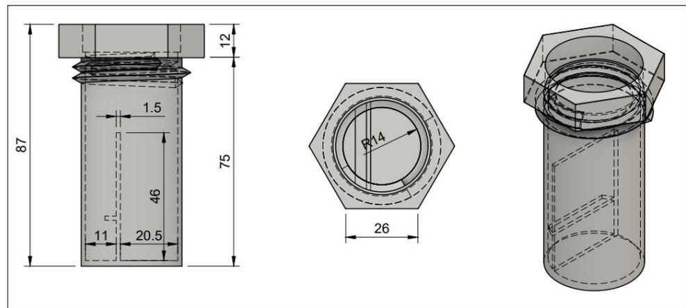
**Figure 14.** Hexagonal shape for the upper part of the inner case.
