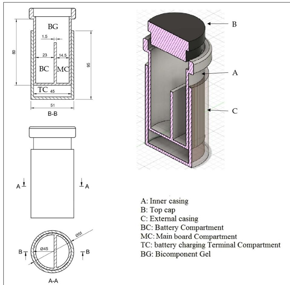
Figure 11. Double-casing assembly.
