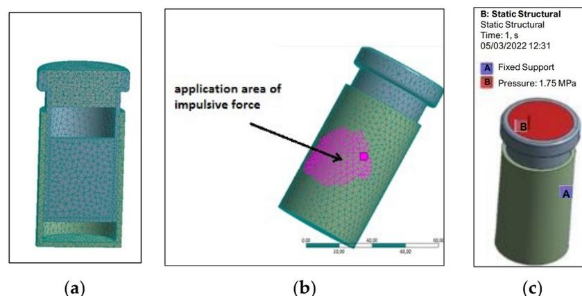
**Figure 7.** (a) Assembly mesh; (b) impulsive force application; (c) distributed force application (Reproduced from [24] with permission from Springer Nature Switzerland AG).
