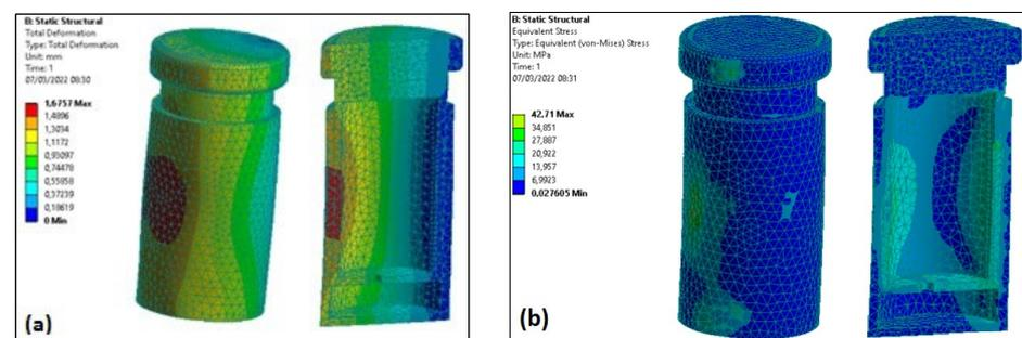
**Figure 8.** (a) Deformation and (b) Von Mises stress under impulsive force (Reproduced from [24] with permission from Springer Nature Switzerland AG).
