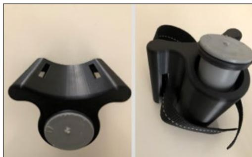
**Figure 5.** Detail of the double curvature surface in the 3D printed version.
