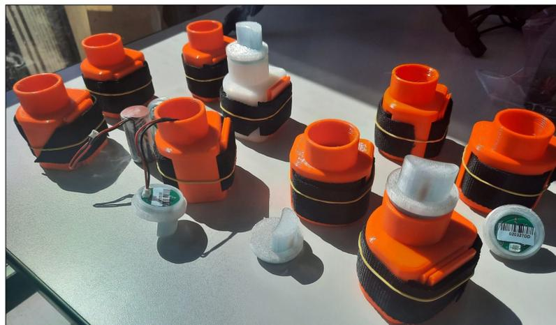
**Figure 6.** Pedometer with reinforced casing, top cap thread and mainboard housed in the cap.
