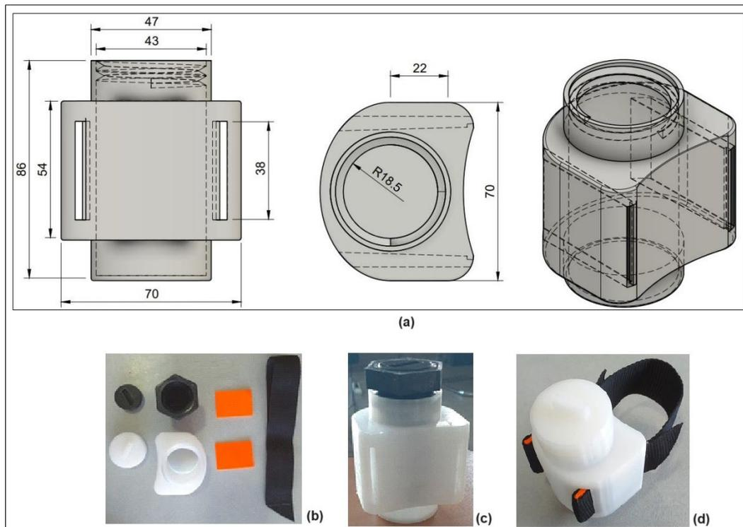
**Figure 16.** Pedometer final model: (a) 3D CAD model of the pedometer; (b) single components and belt; (c) pedometer assembly ready to be attached to the cow leg during the monitoring of oestrus event; (d) pedometer assembly after the pregnancy diagnosis.
