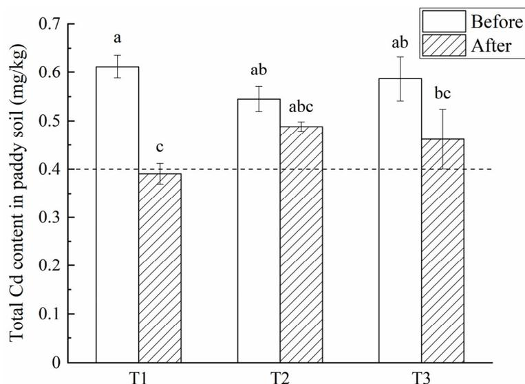
**Figure 3.** Variation in total Cd content in the soil of experimental groups before and after treatment (T3 was control group). Different letters above the error lines indicate significant differences ( $p < 0.05$ ). The dashed line indicates the legal limit of Cd in the agricultural soil (0.4 mg/kg is derived from the Chinese national standard GB 15618-2018).
