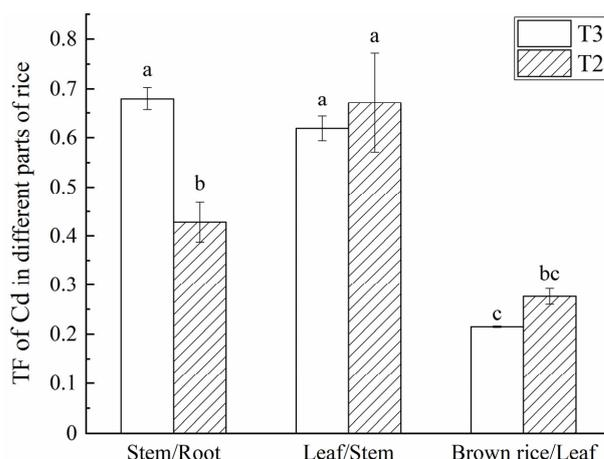
**Figure 6.** Variation in Cd translocation factor in various tissues and organs of rice. The T3 group was the control group, and the T2 group used the geo-electrochemical technology. Different letters above the error lines indicate significant differences ( $p < 0.05$ ).
