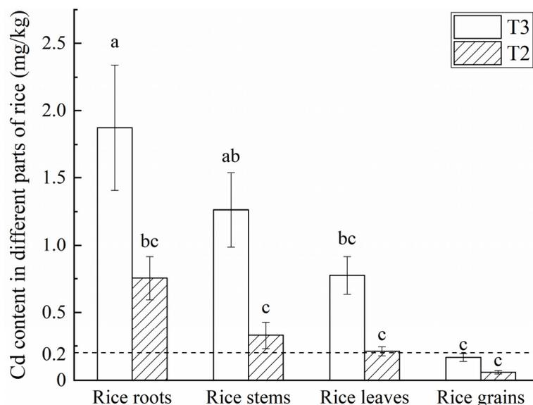
**Figure 4.** Variations in Cd contents in various tissues and organs of rice. The T3 group was the control group, and the T2 group used the geo-electrochemical technology. Different letters above the error lines indicate significant differences ( $p < 0.05$ ). The dashed line indicates the legal limit of Cd in brown rice (0.2 mg/kg is derived from the Chinese national standard GB 2762-2022).
