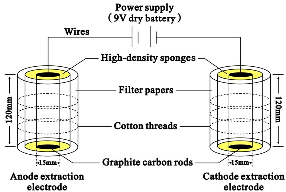
Figure 1. Schematic diagram of the geo-electrochemical technology device.
