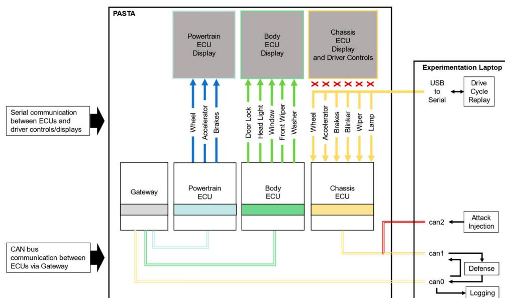
**Figure 2.** Hardware PASTA experimentation environment.
