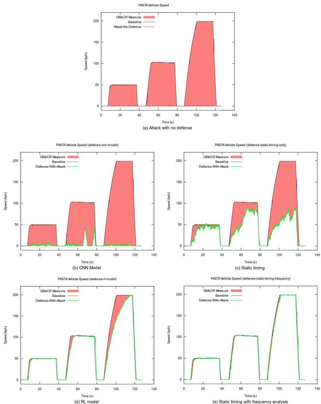
**Figure 6.** Sample graphs of baseline vehicle speed compared to the attack and defenses. Shading shows an approximation of the AUC difference used in the QMoCR measurement. More shading indicates less cyber resilience under the tested scenario.
