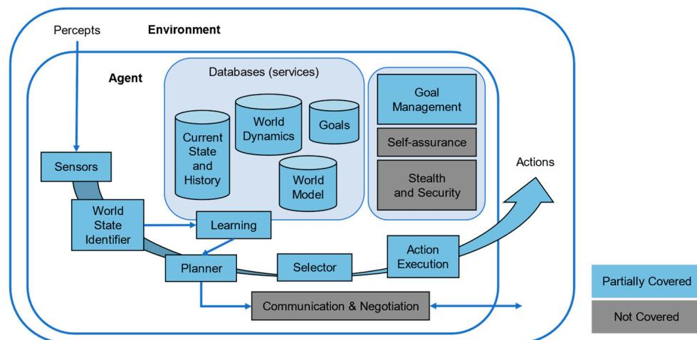
**Figure 1.** The autonomous intelligent cyber-defense agent reference architecture, as used in our prototype, is color-coded to show which pieces are represented.
