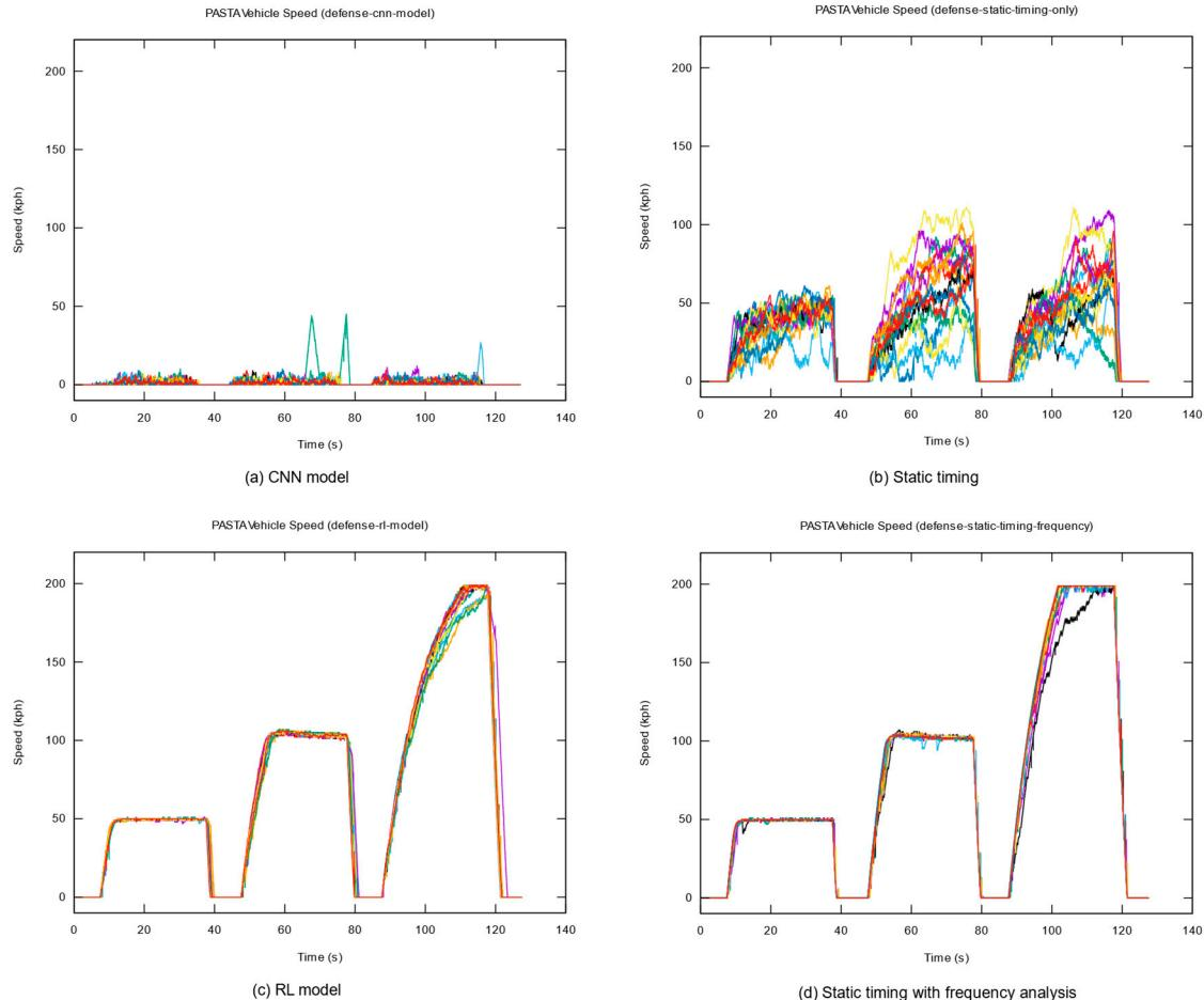
**Figure 5.** Plots of the multiple evaluations run on PASTA hardware per defense while under attack. LSTM is not shown as it was unable to complete a drive cycle due to blocking transmission shifting messages. Colored lines represent unique trials and are plotted to show the variability of each method. The RL model (c) appears as reliable as the hand-crafted oracle method (d).
