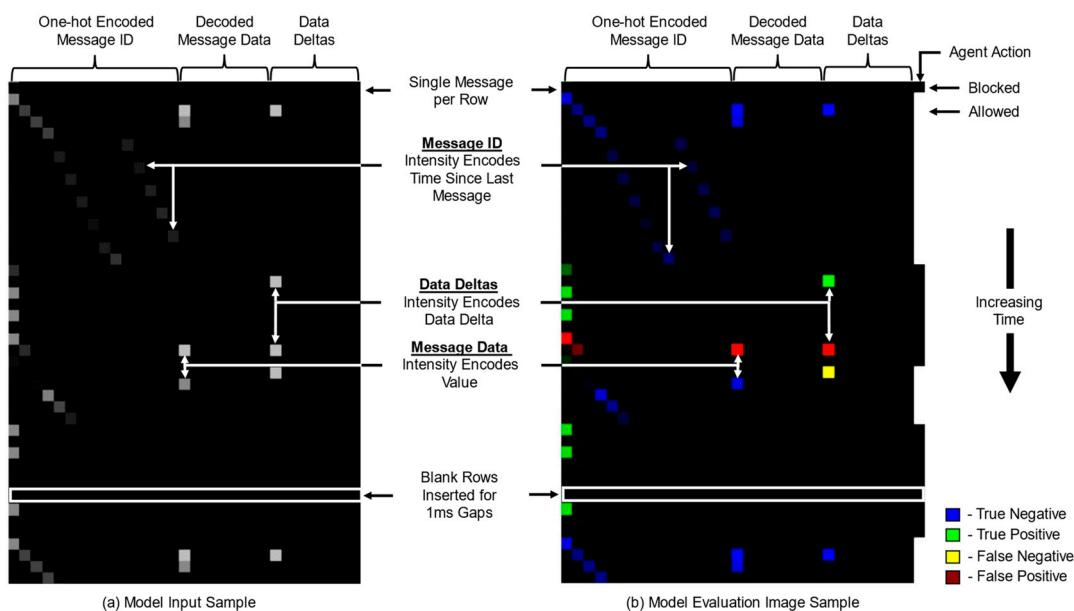
**Figure 3.** (a) Sample grayscale image used as input to defense agent. Each row contains up to 10 highlighted gray pixels that encode the message ID, time delta since the last message of the same ID, message data, and message data delta since the last message of the same ID. (b) Corresponding color representation for human evaluation of the agent learning process during training.
