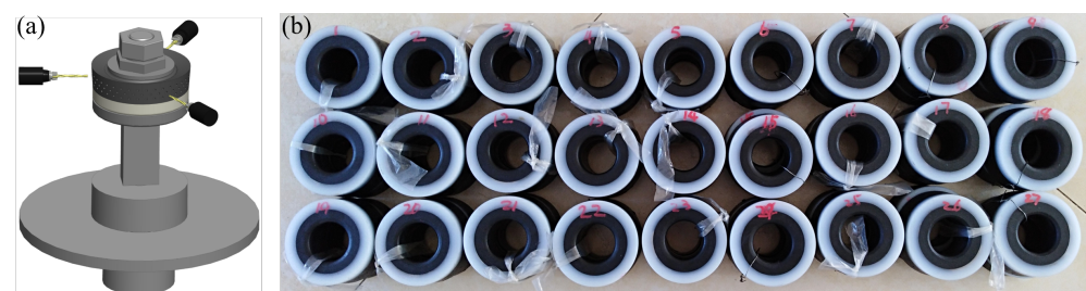
Figure 4. The (a) fabrication and (b) labeling of textured pistons.
