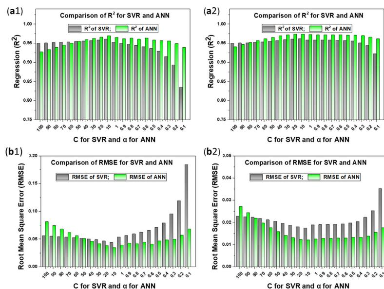
**Figure 11.** Optimization of SVR and ANN models at different C and  $\alpha$  values: (a1,b1) comparative results of predictive models for PR; (a2,b2) comparative results of predictive models for AR.
