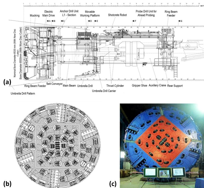
**Figure 6.** Details of TBM 696: (a) tunnelling system, components, and their arrangement; (b) cutterhead with the arrangement of components; (c) TBM 696 photograph.
