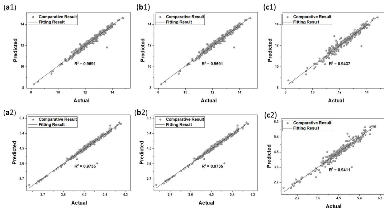
**Figure 16.** Regression analysis based on the actual and predicted TBM values; (a1,b1,c1) represents the penetration rate while (a2,b2,c2) represents the advanced rate for training functions lbfgs, sgd, and ADAM, respectively.
