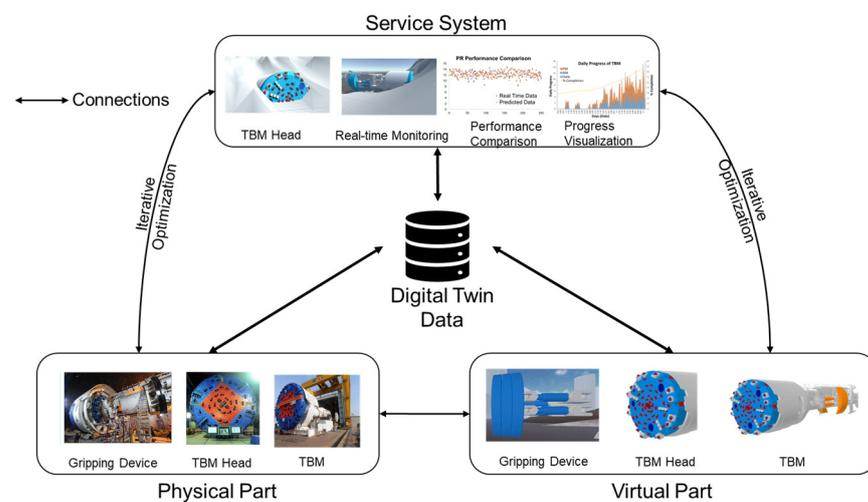
**Figure 1.** Digital twin structure of TBM performance monitoring.
