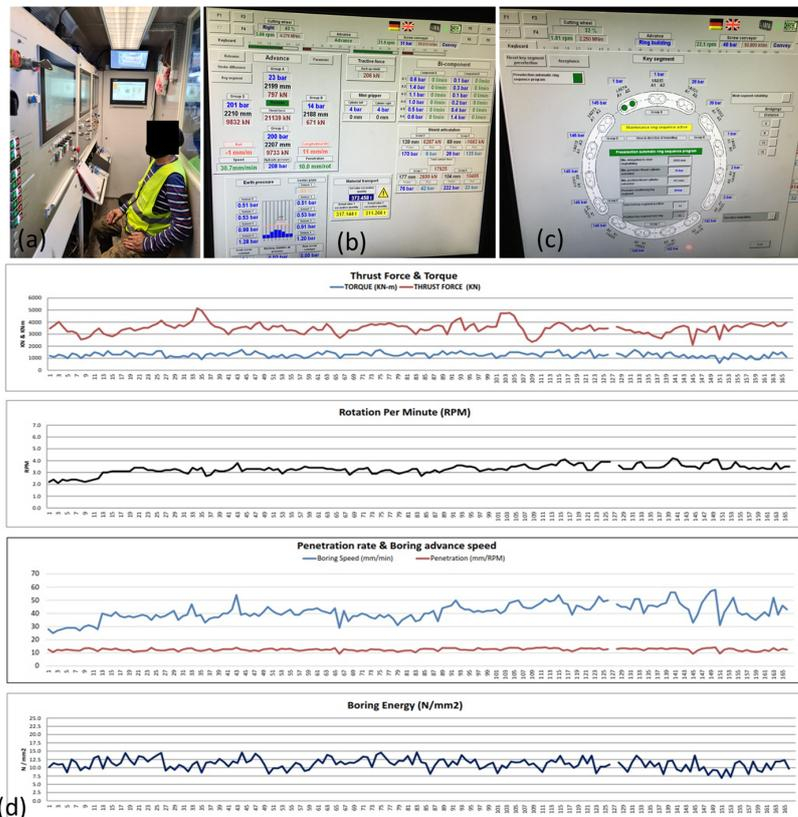
Figure 5. Data collection and TBM input parameter of Neelum Jhelum project: (a) TBM control cabin showing and recording the real-time machine parameters; (b) snapshot of real-time TBM screen showing working machine data; (c) thrust cylinder and rotation motor data; (d) boring data of TBM during operation.
