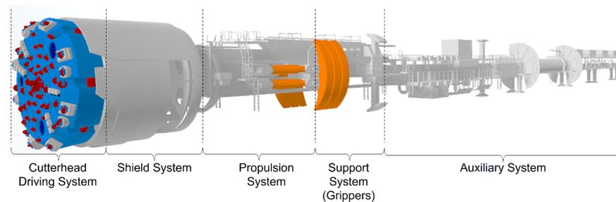
**Figure 8.** Three-dimensional virtual model of a TBM and its components.
