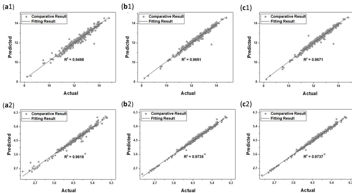
Figure 15. Regression analysis based on the actual and predicted TBM values; (a1,b1,c1) represents the penetration rate while (a2,b2,c2) represents the advanced rate for SVR, ANN, and SVR-ANN models, respectively.
