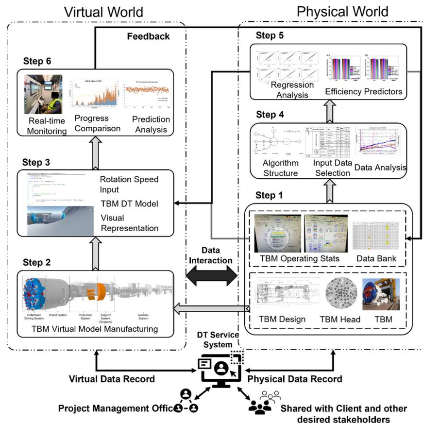
Figure 3. Digital Twin-based framework for TBM performance visualization and monitoring method.
