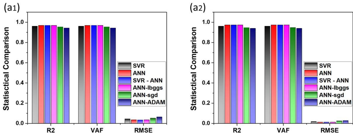
**Figure 17.** Regression analysis based on the actual and predicted TBM values: (a1) comparative results of models for the prediction of penetration rate; (a2) comparative results of models for the prediction of the advance rate.
