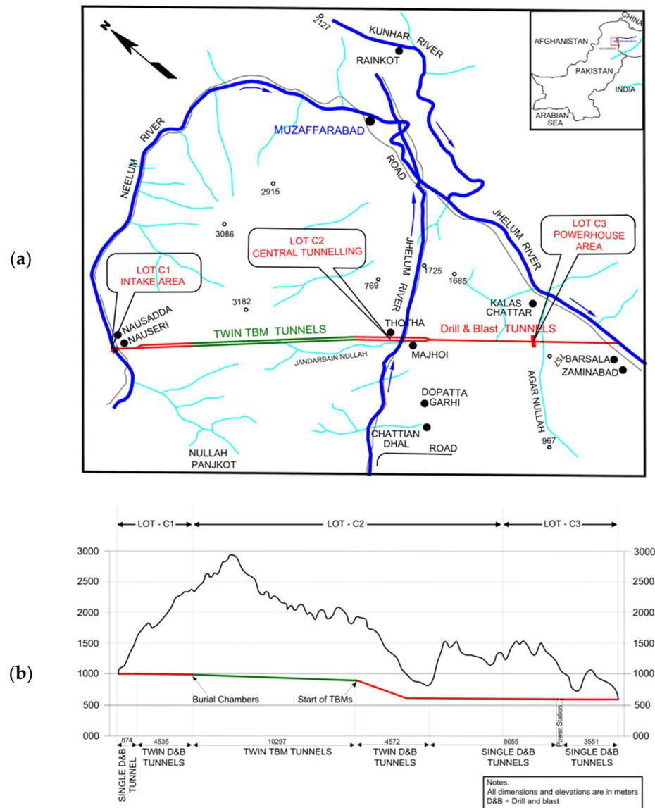
Figure 12. Neelum Jhelum project: (a) layout showing the alignment of TBM twin tunnels and other marked features; (b) terrain profile of the tunnel.
