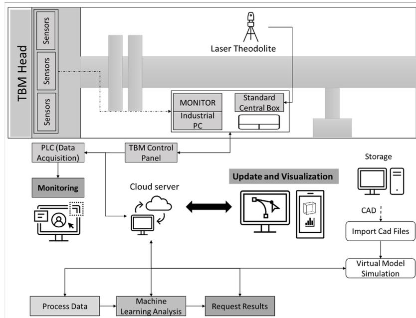
Figure 4. Data transmission from TBM to monitoring.
