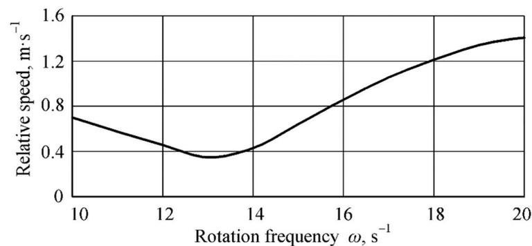
**Figure 5.** Dependence of relative velocity  $\dot{x}$  of haulm particle  $M$  on the angular velocity  $\omega$  of rotation of the thrower (at  $l = 0.1$  m and  $V_n = 35$  m·s<sup>-1</sup>).
