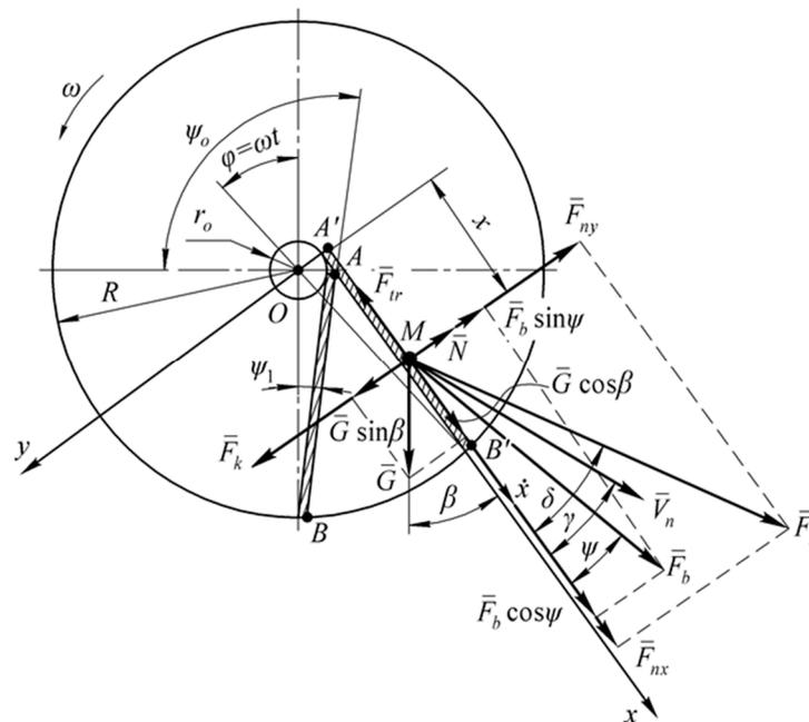
**Figure 2.** Equivalent scheme of haulm particle movement process along the throwing blade surface.
