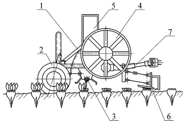
**Figure 1.** Structural and technological scheme of the haulm harvester, with an improved loading mechanism: 1—frame; 2—copying wheel; 3—rotary haulm removing unit; 4—blade thrower; 5—unloading pipe; 6—preliminary root head cutter; 7—drive of the working bodies.
