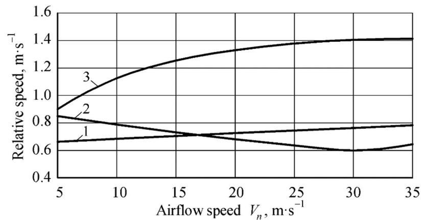
**Figure 4.** Dependence of the relative speed  $\dot{x}$  of the haulm particle  $M$  on the speed of the airflow  $V_n$  and the angular speed  $\omega$  of rotation of the (at  $l = 0.15$  m): 1— $\omega = 10$  s<sup>-1</sup>; 2— $\omega = 15$  s<sup>-1</sup>; 3— $\omega = 20$  s<sup>-1</sup>.
