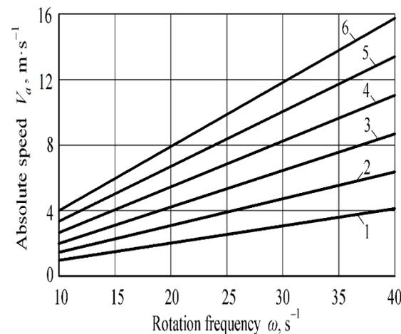
**Figure 3.** Dependence of the absolute speed  $V_a$  of descent of a haulm particle  $M$  from the end of the blade upon the angular velocity  $\omega$  of rotation of the thrower and the length  $l$  of the blade: 1— $l = 0.1$  m; 2— $l = 0.15$  m; 3— $l = 0.2$  m; 4— $l = 0.25$  m; 5— $l = 0.3$  m; 6— $l = 0.35$  m.
