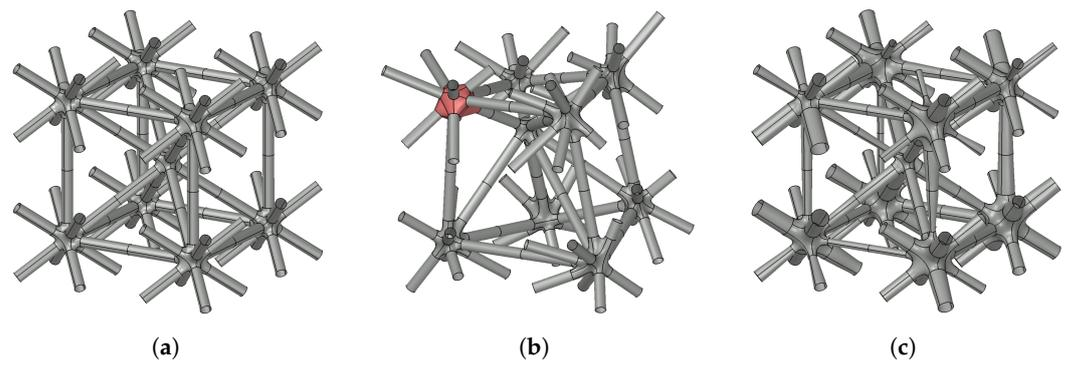
**Figure 10.** Lattice construction algorithm applied for a body-centric cubic elementary cell. (a) Standard version. (b) Randomly shifted nodes. (c) Randomly varied radii.
