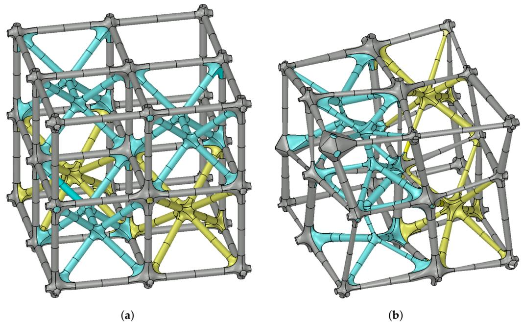
**Figure 11.** Lattice construction algorithm applied for an irregular lattice frame in two configurations. Identical cell topologies are visualised by colour. (a) Standard version. (b) Randomly shifted nodes and randomly varied radii.
