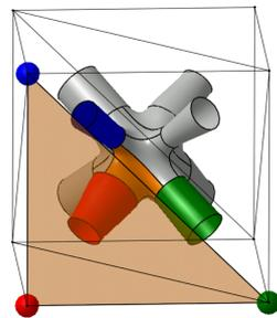
**Figure 6.** Convex hull representation of a node. A triangular face of the convex hull and the corresponding  $G^1$ -continuous 6-patches that is constructed by the lattice algorithm are marked in orange.
