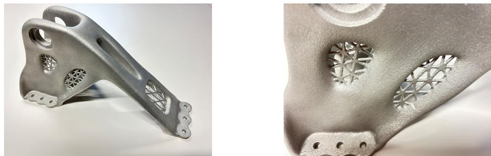
**Figure 12.** (Left): Additively manufactured aircraft component with lattice infills, which are constructed using the discussed method. (Right): Zoom in to lattice infill.
