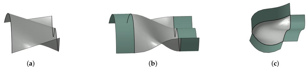
**Figure 1.** Sketches of the three types of surface patches that are required for the lattice construction algorithm developed in this work. (a) Ruled surface. (b)  $G^1$ -continuous ruled surface. (c)  $G^1$ -continuous 3-patch.
