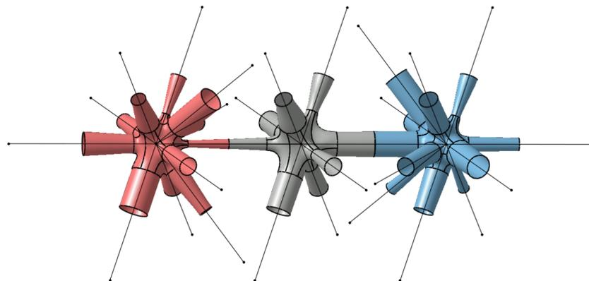
**Figure 4.** Lattice frame with its respective lattice structure. The colouring of the surface patches shows the subdivision of the construction task in single nodes and halves of their corresponding struts.
