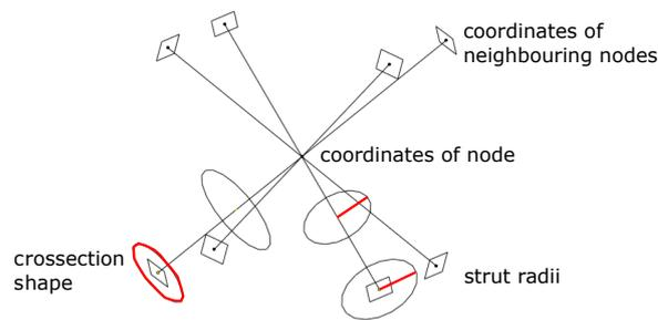
**Figure 3.** Parameters of the lattice structure.
