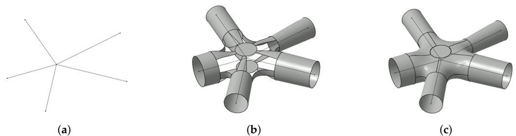
**Figure 7.** Construction stages for nodes with coplanar and almost coplanar edges. The subfigures (a–c) represent the sequence of action.
