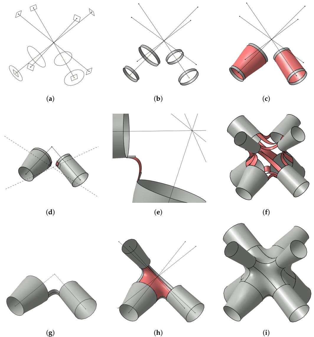
**Figure 5.** Sketches of the most important stages of the general node construction step. The subfigures (a–i) represent the sequence of action.
