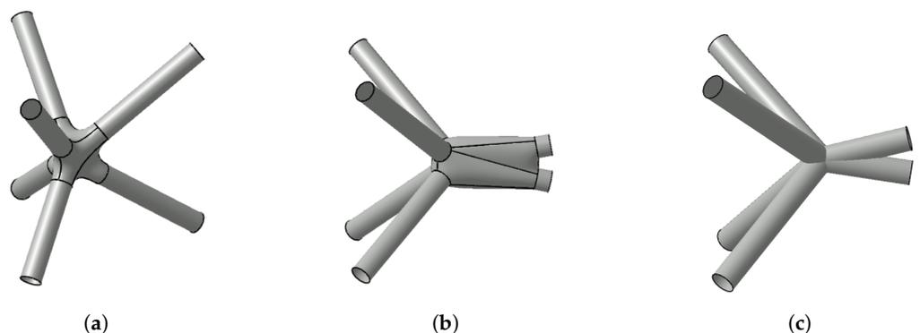
**Figure 9.** Different stages of fallback in geometric continuity due to sharp angles and short struts. (a)  $G^1$ -continuity. (b) Partly fallback to  $G^0$ -continuity. (c) Complete fallback to  $G^0$ -continuity.
