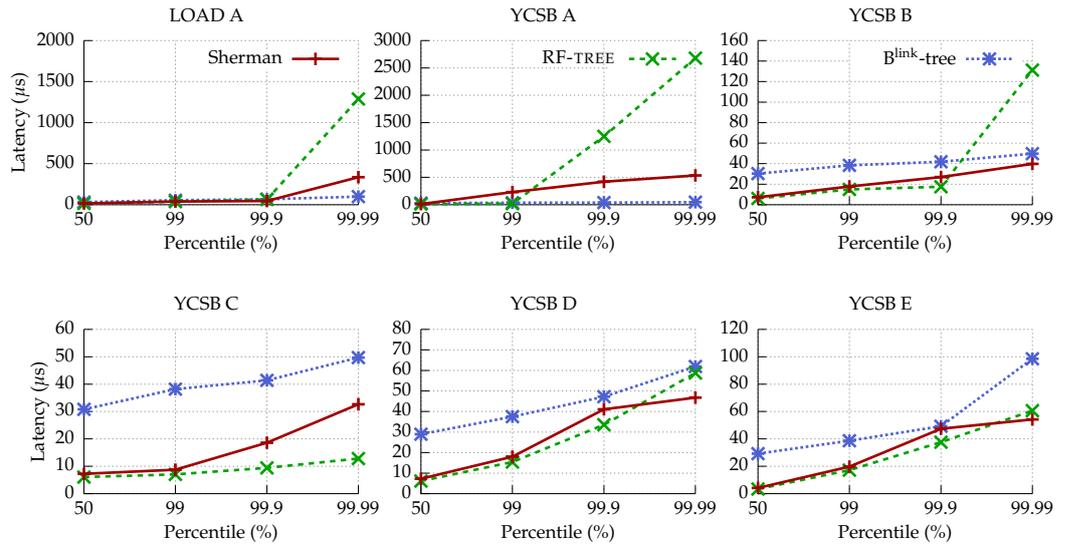
**Figure 9.** Tail latency of range index structures for disagggregated memory with YCSB workload (Zipfian Distribution).
