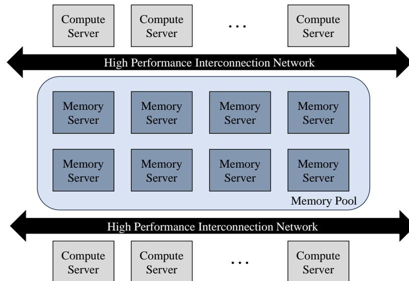
**Figure 1.** Overview of disaggregated memory.
