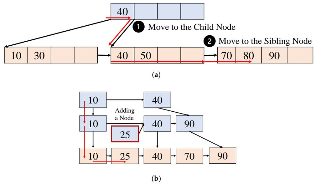
**Figure 2.** Tolerating Transient inconsistency in the concurrent range index structures. (a)  $B^{\text{link}}$ -tree: Example of lookup operation of key 80. When the node split occurs, the reader can tolerate the transient inconsistency by traversing the sibling node. (b) SkipList: Example of lookup operation of key 25. The reader can tolerate transient inconsistency by traversing the lower level when the key is added to the upper level.
