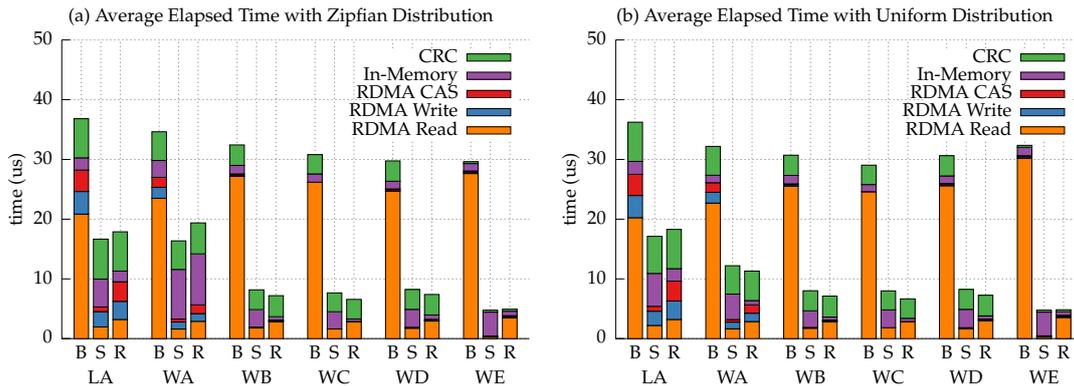
Figure 8. Performance breakdown of range index structures for disaggregated memory with YCSB workload. In this experiment, B stands for B<sup>link</sup>-tree, S stands for Sherman, and R stands for RF-TREE. For workload, LA stands for load A, and WA–WE stand for workload A–E.
