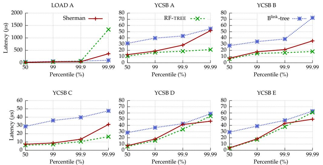
**Figure 10.** Tail latency of range index structures for disagggregated memory with YCSB workload (Uniform Distribution).
