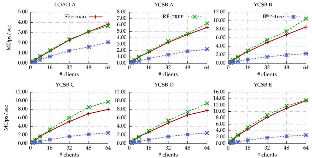
Figure 7. Throughput of range index structures for disaggregated memory (uniform distribution).
