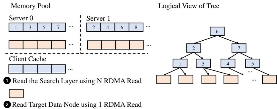
**Figure 3.** Overview of RF-TREE. When the SLC is empty, the client reads the search layer from the memory servers. When the search layer is cached and built, the client finds the address of the target data node. Using the address, the client reads the data node. In the figure, N is the number of the server.
