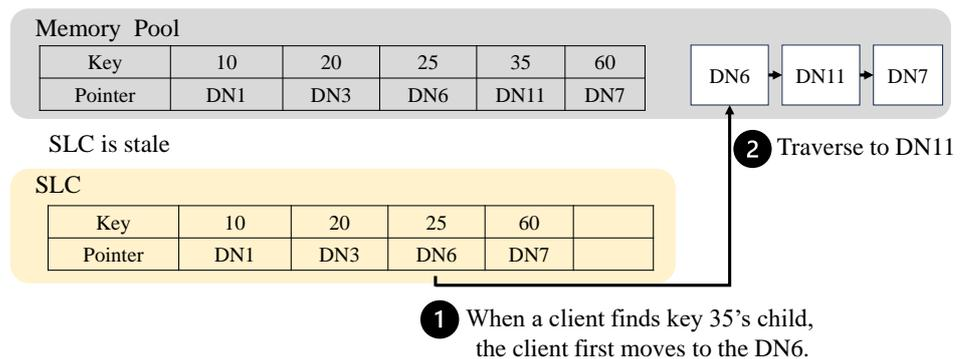
**Figure 5.** An example of a stale SLC. ① A client moves to the child node when it finds a key that is larger than the target key. ② The client traverses the child nodes to find the target key.
