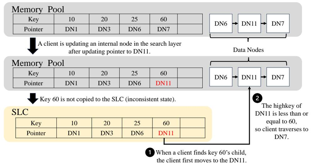
**Figure 4.** An example of an inconsistent search layer. When RF-TREE updates a node, RF-TREE writes a pointer (value) and then writes the key. ① Since DN11 has smaller keys than DN7, ② the client moves to the DN7.
