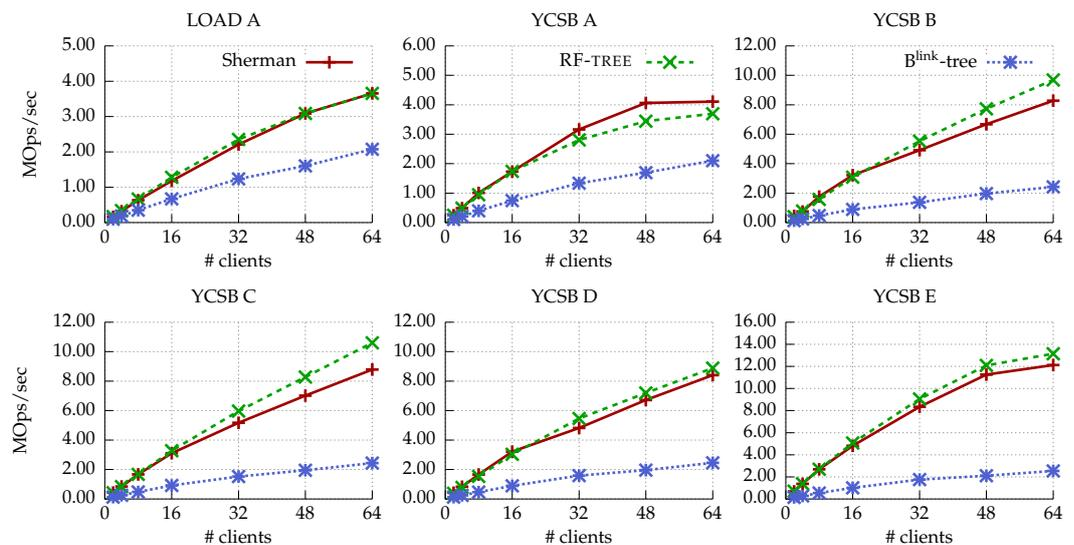
Figure 6. Throughput of range index structures for disaggregated memory (Zipfian distribution).
