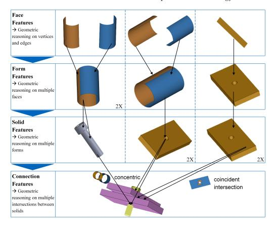
**Figure 3.** Different levels of features, from simple face features to connection features, relevant to assembly processes.
