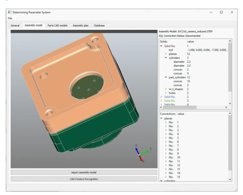
Figure A4. The results (recognized solid features and intersections) of the use case.
