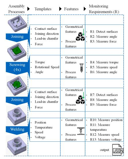
Figure 5. Use case – identification of monitoring features of an assembled surround view camera.
