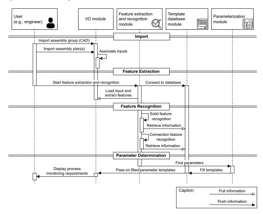
**Figure 2.** The sequence diagram shows the interactions between the modules for automatic identification of process monitoring characteristics and the user. The user role and modules are shown in Figure 1 and provide additional information about which data must be selected and imported and how the results can be retrieved. Additionally, the individual phases can be seen, such as *Import*, *Feature Extraction, Feature Recognition*, and *Parameter Determination*.
