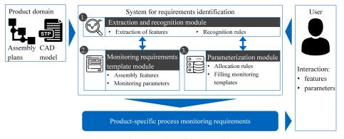
**Figure 1.** System overview for the identification of process monitoring requirements in assembly products.
