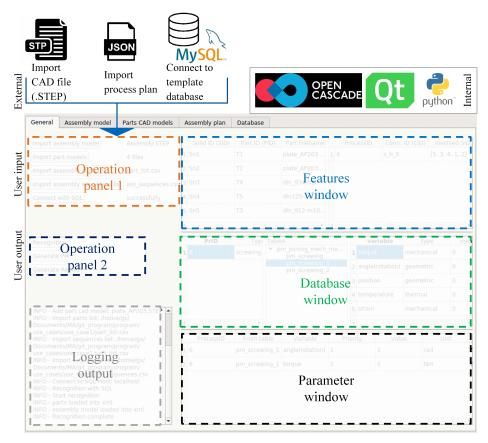
**Figure 4.** Graphical user interface for the detection and visualization of assembly features relevant to monitoring.
